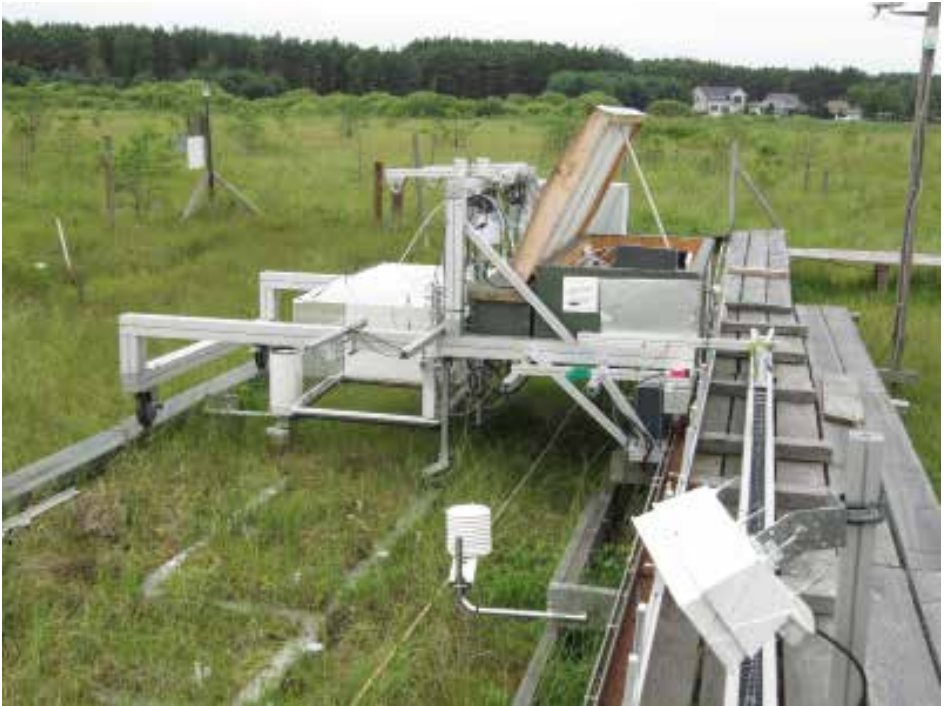
Photo 87: An automatic measuring station for the balance of greenhouse gasses, a manipulation experiment in Rześcińskie Mire (photo by J. Kujawa-Pawlaczyk).
