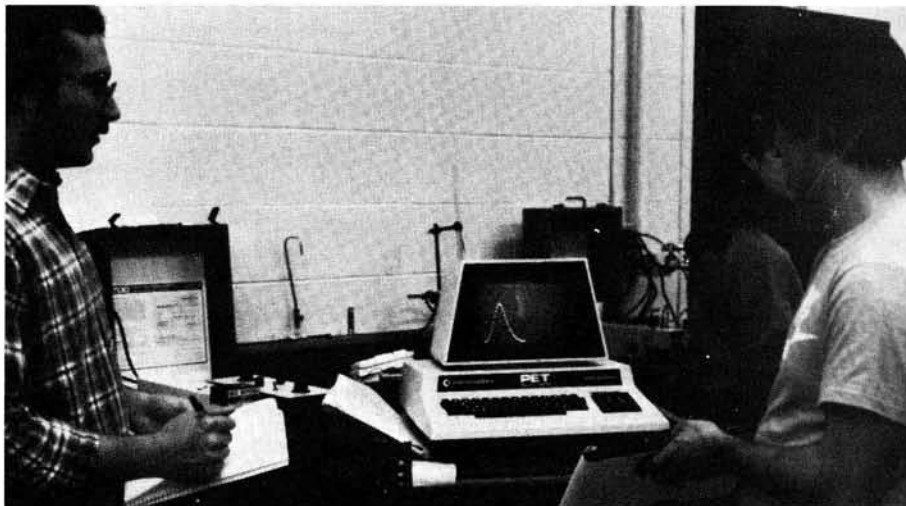
Chemical Engineering students using a computer interfaced to a gas chromatograph. The students use gas chromatographs to analyze mixtures of chemicals. The computer is used both to acquire and analyze the data. Using the computer saves hours over conventional methods.
