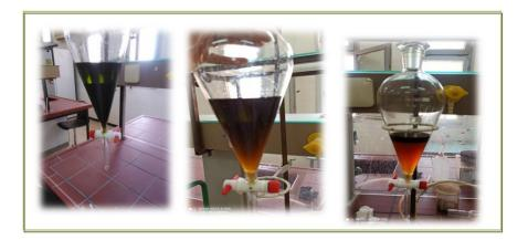
Figure.II.9: Liquide-liquide extraction process.
