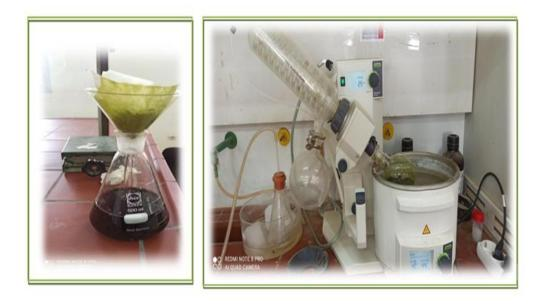
Figure.II.8: Filtration and evaporation process.
