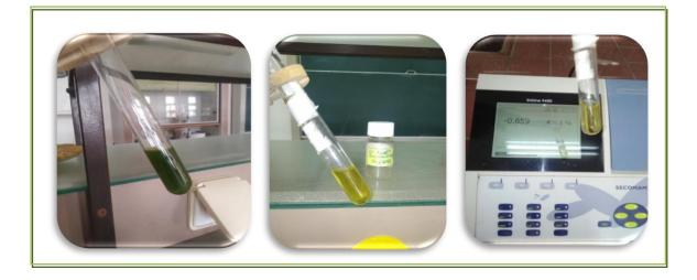
Figure .II.18 : Samples before and after incubation for determination of anti oxidant activity of EtOAc extract of *B.Bituminosa*.
