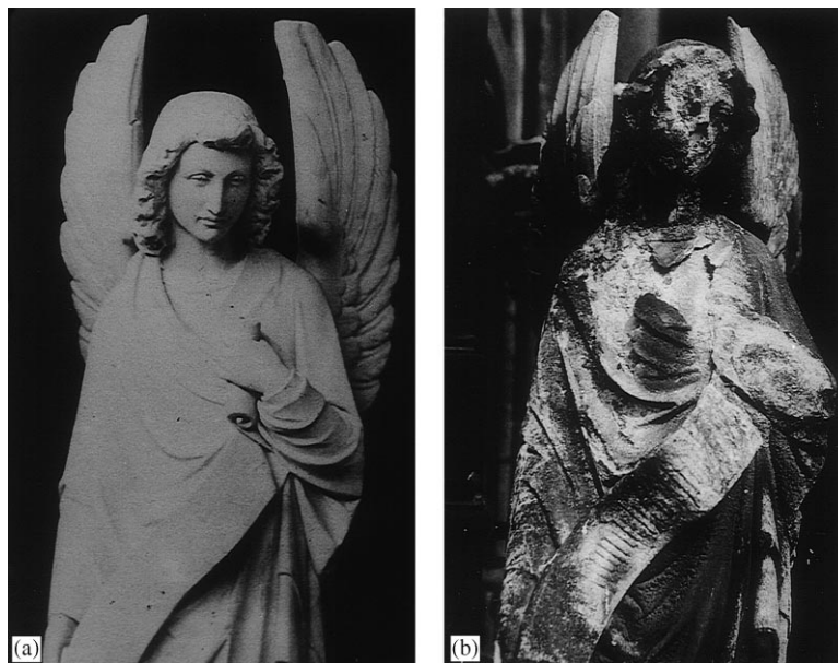
Fig. 1. Influence of biodeterioration processes on an angel statue at the “Peters”-Portal on the cathedral of Cologne (Germany); documented by the original object in 1880 ((a) photograph by Anselm Schmitz, Cologne) and the respective weathered statue in 1993 ((b) photograph by Dombaumeister Prof. Dr. A. Wolff, Cologne).
