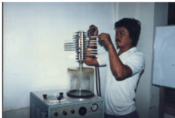
Figure 11. The pollen ampoules being tested for vacuum leak using a spark tester
