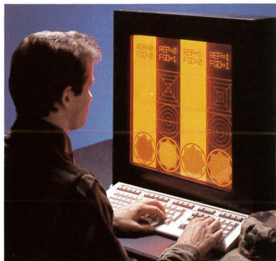
1024 x 1024 pixels 100 lines of 160 characters 12 x 12 to 17 x 17 inches 19 inch rack mountable
