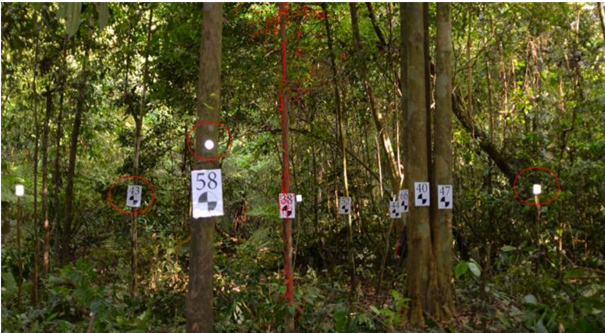
Figure 3-4: Shown the tagged trees, overlaid cloud points, set up of cylindrical and circular retro-reflectors
