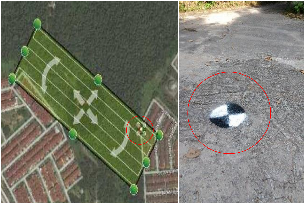
Figure 3-6: The UAV flying (left) and GCP's maker (right)
