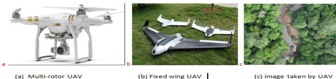
Figure 1-3: The two categories of UAV system and sample of UAV image
