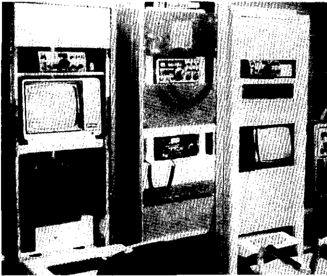
The HF spread-spectrum station at K8MMO. A Xerox 820 computer was used for control. The transmit position is on the right; receive is on the left.
