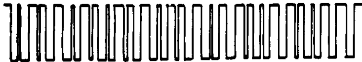
Fig 3—A DSSS carrier is shown at the jumper between the transmitter (output of U8D) and receiver. The scanning rate is 1 \mu s/div.
