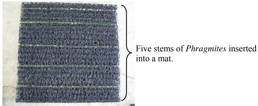
Fig. 2 Drain mat used to make artificial floating islands for water purification
