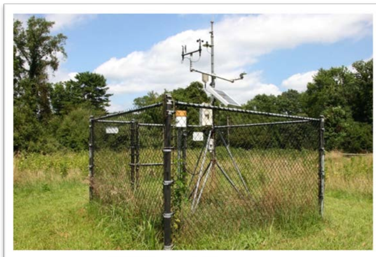
Weather station in Howell Township at 40.192056, -74.196238. Photo credit: J. Dodds
