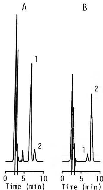
Figure 2. LC chromatograms of mixture of 1.0 \mu\text{g}/\text{mL} of paraquat dichloride (1) and diquat dibromide (2). A, detection at 257 nm; B, detection at 310 nm.
