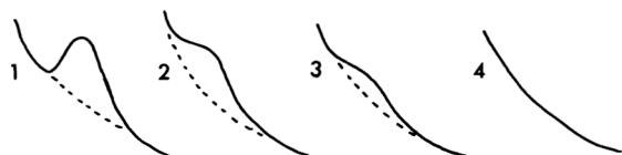
Figure 9. Classification of UV spectrometric peaks: 1, a distinct peak in the spectrum, quantitative calculation without problem; 2, a peak is present, but not quantitatively calculable; 3, a very weak slope is present; 4, no deviation from a blank is observed.
