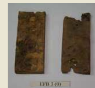
Sampel tanpa Borogard ZB selepas 16 minggu didedahkan kepada anai-anai Sample without Borogard ZB after 16 weeks of termite exposure test in the field
