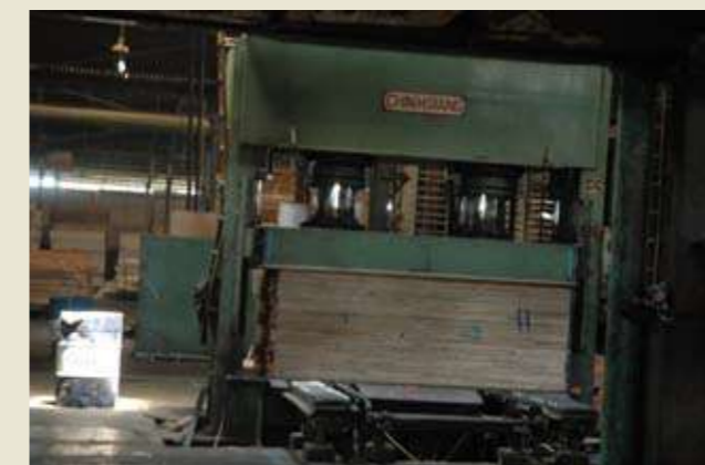
Pra-penekanan ke atas papan lapis OPT Pre-press of OPT plywood
