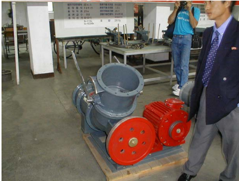
Figure 8-1: DPRK-made Mini-Hydroelectric Turbine-Generator 206
