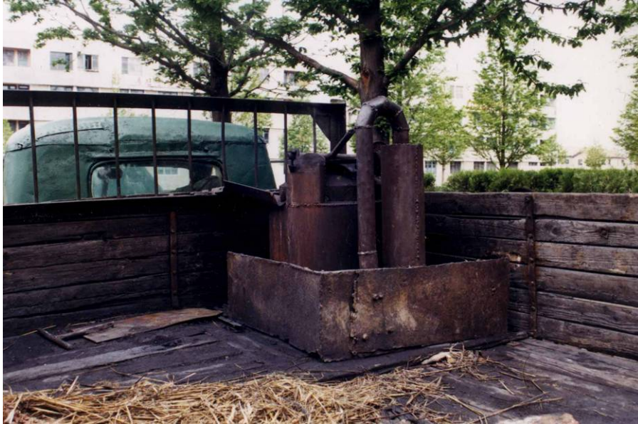
Figure 2-24: Photo of DPRK Truck Powered by a Coal (and/or biomass) Gasifier 134
