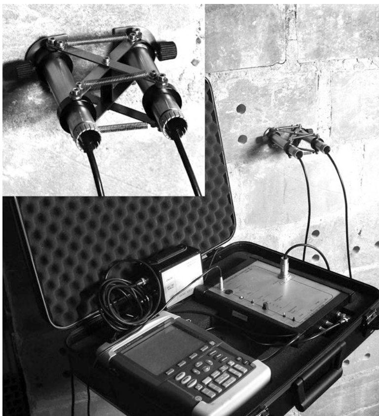
Fig. 8.5 Double-probe ultrasonic device for in-depth parallel to surface measurements
