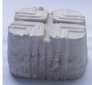
Fig. 10.2 The aspects of stucco models under different external factors. (a) Stucco treated with \text{Na}_2\text{SO}_4 and kept at 25 °C ( t = 0 ), (b) stucco treated with \text{Na}_2\text{SO}_4 and kept at 25 °C ( t = 8 days), (c) stucco treated with NaCl at 5 °C ( t = 0 ), (d) stucco treated with NaCl at 5 °C ( t = 8 days), (e) stucco treated with NaCl at 25 °C ( t = 8 days), (f) stucco treated with NaCl at 50 °C ( t = 8 days)
