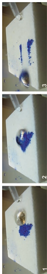
Fig. 1.8 The self-/easy cleaning property of a water-repellent coating deposited on marble is demonstrated in these successive snapshots. The coating was prepared using a waterborne silane/siloxane product (Silres BS 4004) and silica nanoparticles; the nanoparticle/siloxane mass ratio was 0.2. The coated surface of the marble segment was intentionally contaminated with a blue pigment. Water drops that were left to roll off removed the pigment particles. A sequence number (1–3) is provided in the lower left corner of each photograph. Reprinted with permission from reference number [23], Copyright (2013), John Wiley & Sons, Inc
