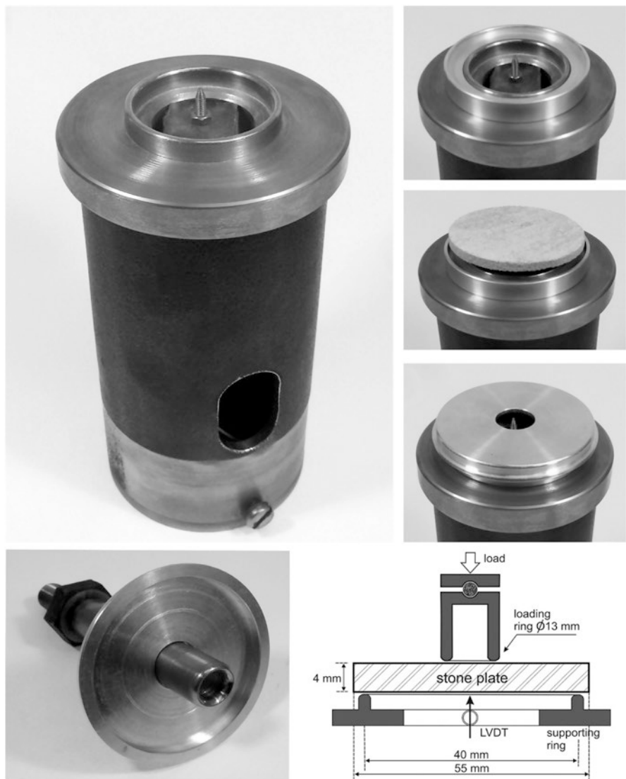
Fig. 8.3 Testing rig for biaxial bending—schematic sketch (bottom right), sequence of composition (upper pictures, left supporting ring, right disc alignment ring, stone disc in the alignment ring, load—hollow piston—alignment ring)
