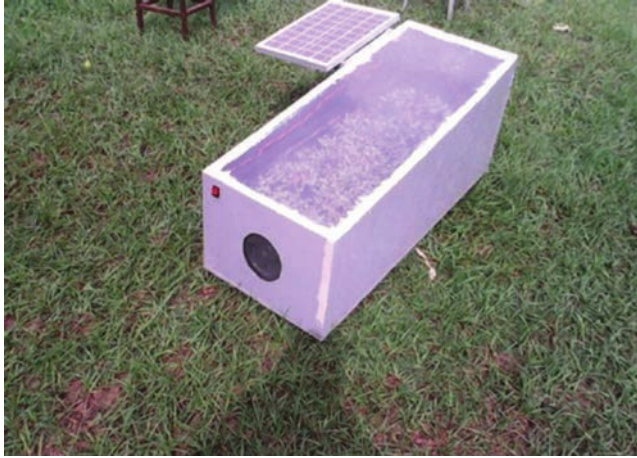
Fig. 8.4. Solar drying of chester leaves in a trough.
