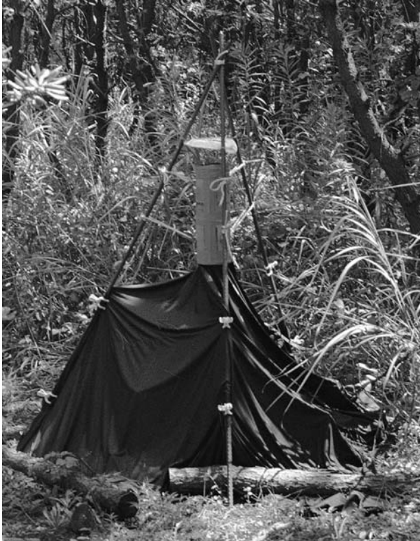
Fig. VI.16 An “automatic contaminating device” for releasing Beauveria -contaminated Cryphalus fulvus adults
