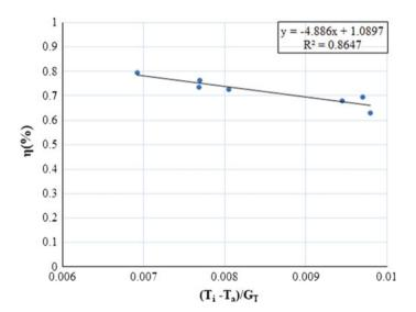
**Fig. 3**  $\eta$  (%) versus  $(T_i - T_a)/G_T$  graph for 32° tilt angle
