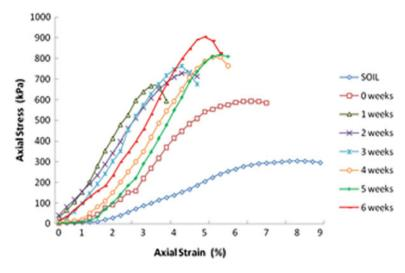
Fig. 11 UCC curves showing variation in strength of terrazyme-treated marine clay on curing
