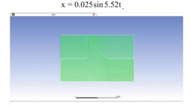
Fig. 16 Meshed finite element model of the Koyna dam in FLUENT
