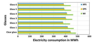
Fig. 4 Annual electricity consumption for cooling with EPS, XPS, and without insulation (WI) for Barmer city
