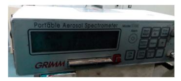
Fig. 3 Portable aerosol spectrometer for PM measurement
