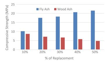
Fig. 2 Compressive strength of bricks
