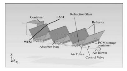
Fig. 4 Schematic diagram of the V-trough solar air heater [13]
