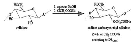
Fig. 1 Reaction scheme of the carboxymethylation of cellulose
