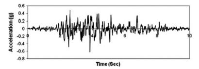
Fig. 6 Koyna longitudinal earthquake motion
