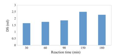
Fig. 9 Effect of various reaction periods of SMCA on degree of substitution of CMC from fungal tea biomass
