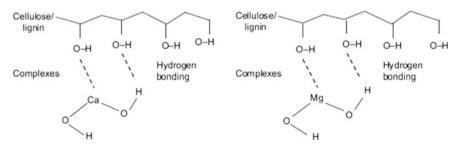
Fig. 1 Chemical structure of Ca(OH)<sub>2</sub> and Mg(OH)<sub>2</sub> modified fibres [4]
