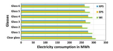
Fig. 3 Annual electricity consumption for cooling with EPS, XPS, and without insulation (WI) for Bengaluru city
