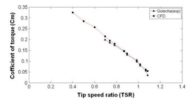
Fig. 5 Variation of moment coefficient ( $C_{\rm m}$ ) against tip-speed ratio ( $\lambda$ )
