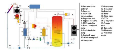
Fig. 1 Schematic diagram of the test rig [10]
