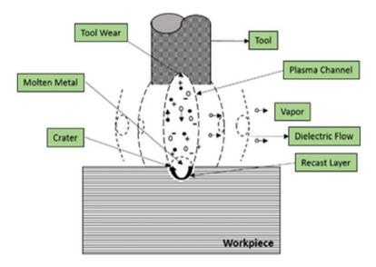
Fig. 2 EDM process mechanism
