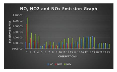
Fig. 5 NO, NO<sub>2</sub>, and NO<sub>x</sub> emissions during the EDM process
