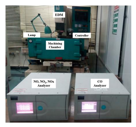
Fig. 3 ELEKTRA 5535 ZNC EDM with NO<sub>x</sub> and CO analyzers
