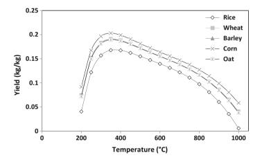
Fig. 2 Effect of pyrolysis temperature on water yield from different straw biomass
