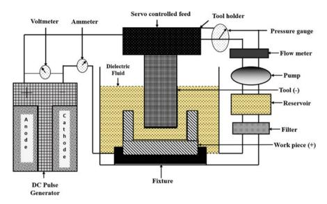
Fig. 1 A schematic diagram of the EDM process
