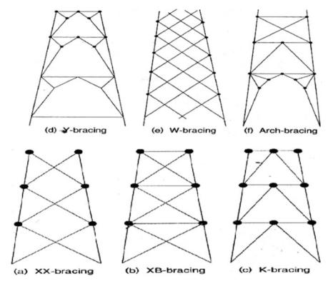
Fig. 2 Different types of bracings
