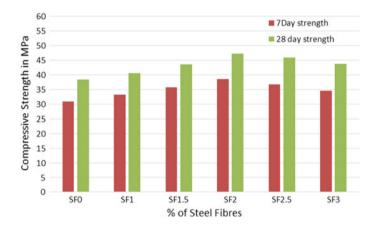
Fig. 2 Effect of fiber percentage on compressive strength
