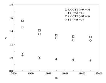
Fig. 8 Comparison of TPF for R-CCTT and TT
