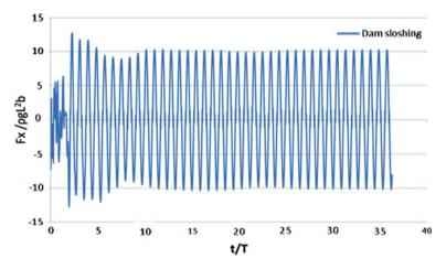
Fig. 17 Time history of lateral force exerted by fluid on dam face
