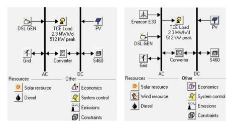
Fig. 6 HOMER simulation model of hybrid configurations
