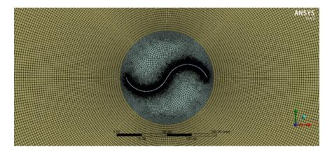
Fig. 2 Rotating circular region with Savonius blade
