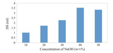
Fig. 8 Effect of various concentrations of NaOH on degree of substitution of CMC from fungal tea biomass
