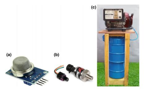
Fig. 5 a Gas leakage sensor, b pressure sensor, c Portable Bio-electric Plant
