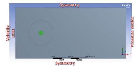
Fig. 1 Modeling of Savonius turbine
