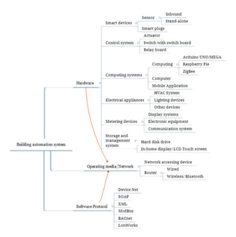
Fig. 4 Components of a typical BAS module
