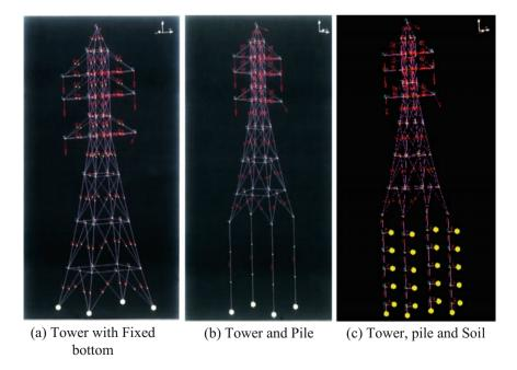
Fig. 4 Analysis cases of the study. a Tower with fixed bottom, b tower and pile, c tower, pile, and soil
