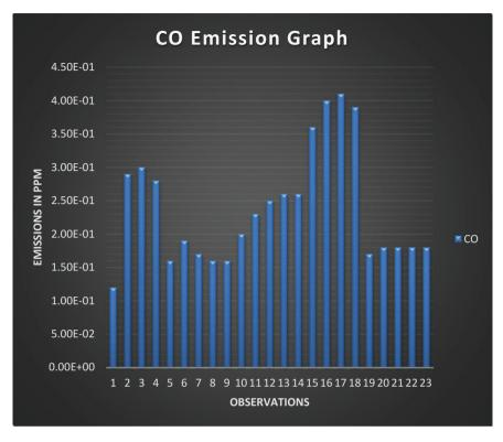
Fig. 6 CO emission during the EDM process
