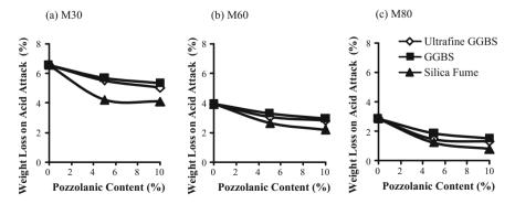
Fig. 11 Effect of addition of low energy cement replacement materials on acid attack resistance
