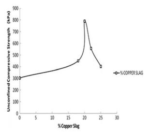
Fig. 7 UCC curves showing variation in strength of lime mixed copper slag-treated marine clay on curing
