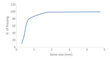
Fig. 1 Sieve analysis of M-sand
