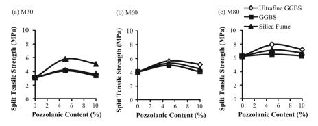
Fig. 8 Effect of addition of low energy cement replacement materials on split tensile strength
