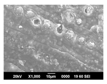
Fig. 3 SEM analysis of CaCl<sub>2</sub> modified coir fibre
