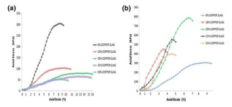
Fig. 5 a Stress-strain curves of marine clay treated with copper slag. b Stress-strain curves of marine clay treated with copper slag and 5% lime
