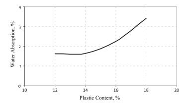
Fig. 7 Variation of water absorption of concrete blocks with varying % of plastic content
