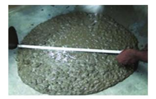
Fig. 3 Slump flow test
