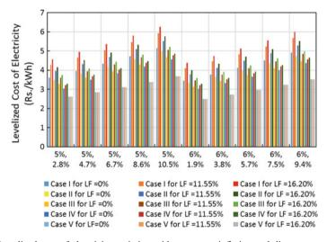
Fig. 7 Levelized cost of electricity variation with respect to inflation and discount rate
