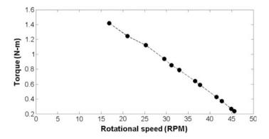
Fig. 6 Variation of torque with rpm of turbine
