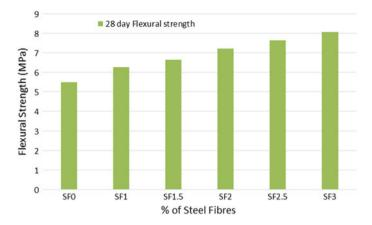
Fig. 3 Effect of fiber percentage on flexural strength
