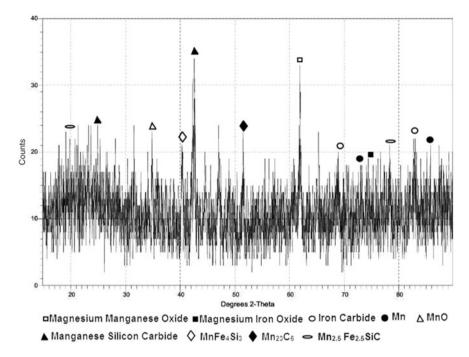
Fig. 4 XRD analysis of sample reduced at 1250 °C (20% LECO, pellet)
