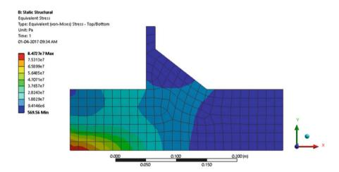
Fig. 21 Equivalent stress of the dam
