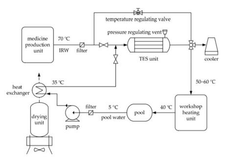
Fig. 8 System configuration of a workshop heating system [20]
