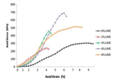
Fig. 1 Stress-strain curves of marine clay treated with different percentages of lime
