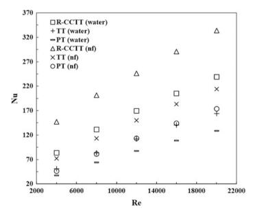
Fig. 5 Comparison of Nu with water and nanofluid for PT, TT, and R-CCTT (y/W = 5)
