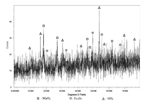
Fig. 1 XRD analysis of manganese ore
