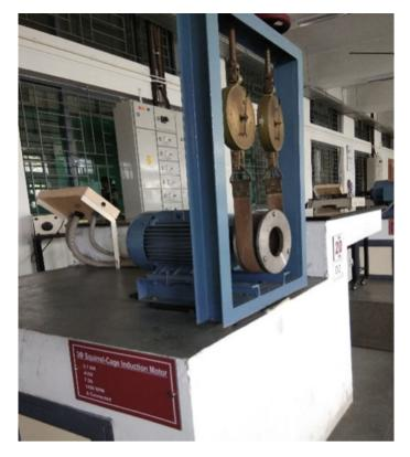
Fig. 2 Testing equipment to conduct load test on three-phase 5 HP induction motor
