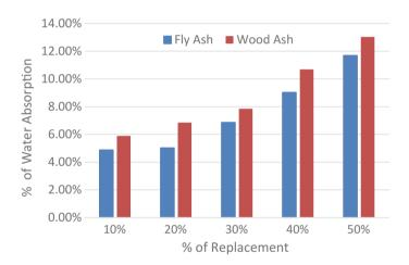
Fig. 3 Water absorption of bricks
