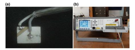
Fig. 2 a High-frequency PZT, b impedance analyzer (LCR meter)
