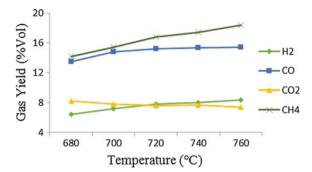
**Fig. 3** Variation of product gases in air–steam gasification with temperature at ER = 0.32 and SBR = 0.66
