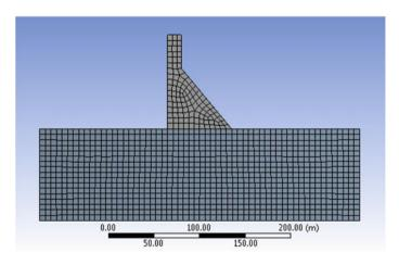
Fig. 5 Meshed model of Koyna dam considering SSI
