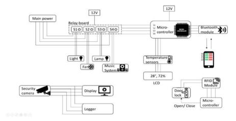
Fig. 7 Schematic circuit diagram of the RRA Module
