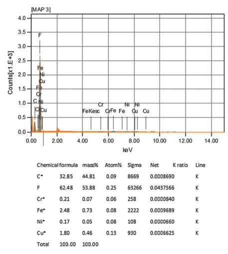
${f Fig.\,6}$  EDS image showing the materials deposited on the spectrometer filter after the EDM process
