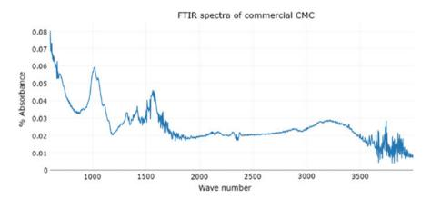
Fig. 4 FTIR spectrum of commercially available carboxymethyl cellulose
