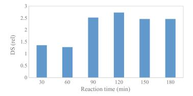
Fig. 5 Effect of reaction period of NaOH on degree of substitution of CMC from fungal tea biomass
