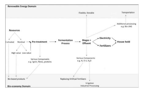
$\textbf{Fig. 6} \hspace{0.2cm} \textbf{Schematic diagram of potential technical connections between biogas renewable energy and bio-economy domains}$
