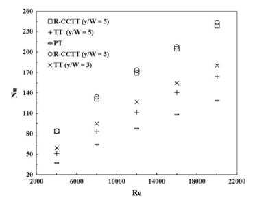
Fig. 4 Comparison of Nusselt number (Nu) for R-CCTT with TT and plain tube
