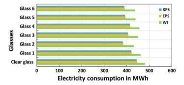
Fig. 6 Annual electricity consumption for cooling with EPS, XPS, and without insulation (WI) for Thiruvananthapuram city
