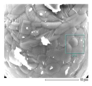
Fig. 5 Pellet with 10% pet coke reduced at 1200 °C
