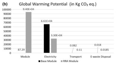
Fig. 11 a Abiotic depletion of base module versus RRA module. b Global warming potential of base module versus RRA module
