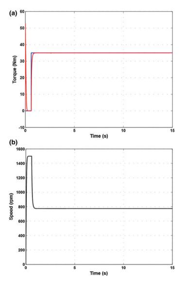
Fig. 3 a Torque in the first 15 s of starting a six-phase induction motor.  $\bf b$  Speed in the first 15 s of starting a six-phase induction motor
