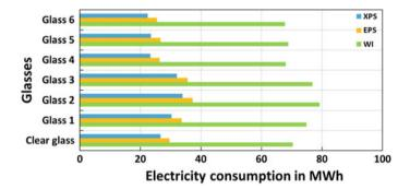
Fig. 8 Annual electricity consumption for heating with EPS, XPS, and without insulation (WI) for Srinagar city
