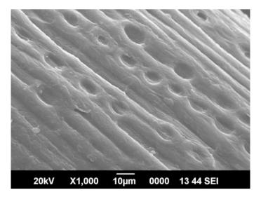
Fig. 2 SEM analysis of unmodified coir fibre
