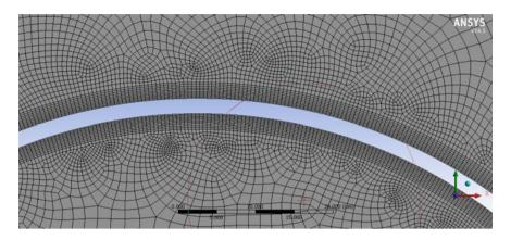
Fig. 3 Inflation meshing in the vicinity of blade surface
