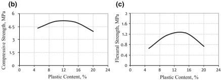
Fig. 4 a Solid concrete blocks mixed with granulated plastic casted in varying mixes, and variation of b compressive and c flexural strength of bricks with varying plastic content
