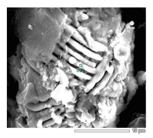
**Fig. 9** Pellet with 20% LECO reduced at 1250 °C
