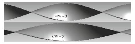
Fig. 1 Continuous rectangular cut twisted tape (R-CCTT) inserts with twist ratio 5 and 3
