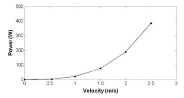
Fig. 7 Variation of power with respect to flow velocity
