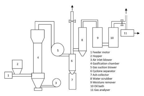
Fig. 1 Experimental setup of the bubbling fluidized bed gasifier
