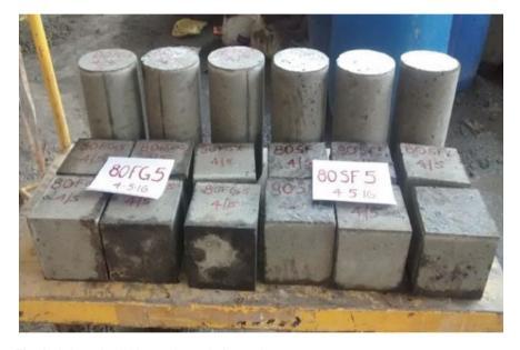
Fig. 4 Cube and cylinder specimens before curing
