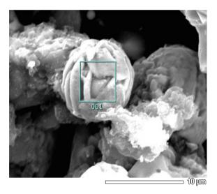
**Fig. 7** Briquette with 20% pet coke reduced at 1250 °C
