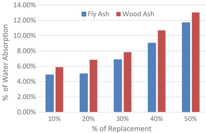
**Fig. 3** Water absorption of bricks
