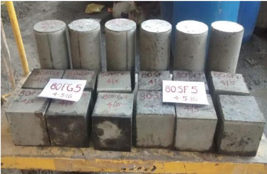
**Fig. 4** Cube and cylinder specimens before curing
