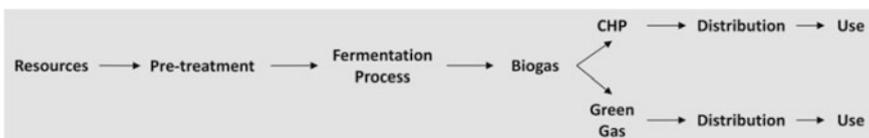
**Fig. 1** Schematic representation of a typical biogas production process
