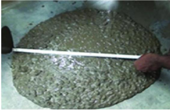
**Fig. 3** Slump flow test
