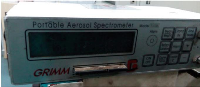
**Fig. 3** Portable aerosol spectrometer for PM measurement
