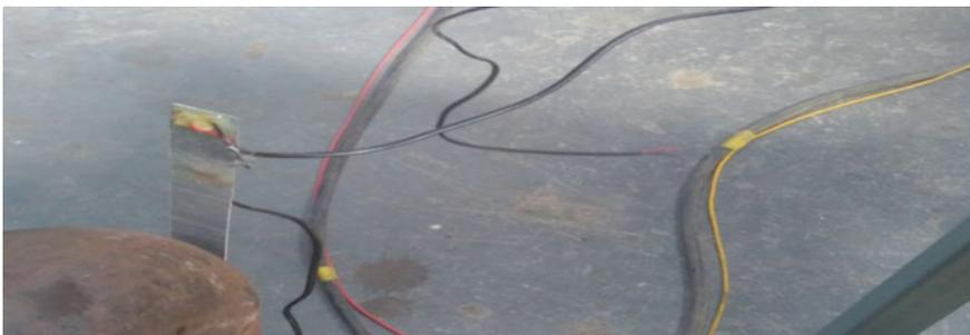
**Fig. 1** PZT connected to structure through aluminum foil
