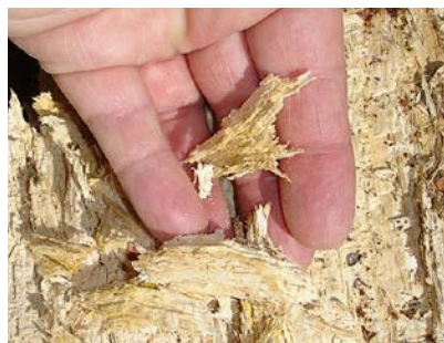
Figure 7.96. Wood decayed by a white rot pathogen. Decayed wood feels soft and spongy and appears stringy and bleached. B. HAGEN
