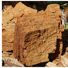
Figure 7.97. Brown rot caused by sulfur fungus ( Laetiporus gilbertsonii ) in black oak. In the advanced stage of infection, wood affected by the pathogen is dry, rusty brown, crumbly, and blocky. B. HAGEN
