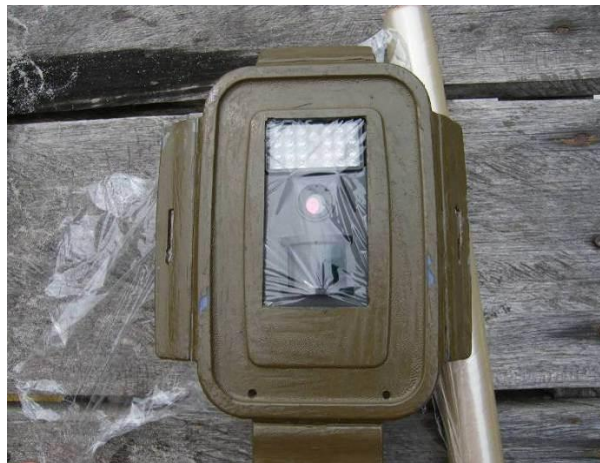
Figure 8-6 Bushnell protected against humidity and external damage by a Tupperware box containing silica with cling film.
