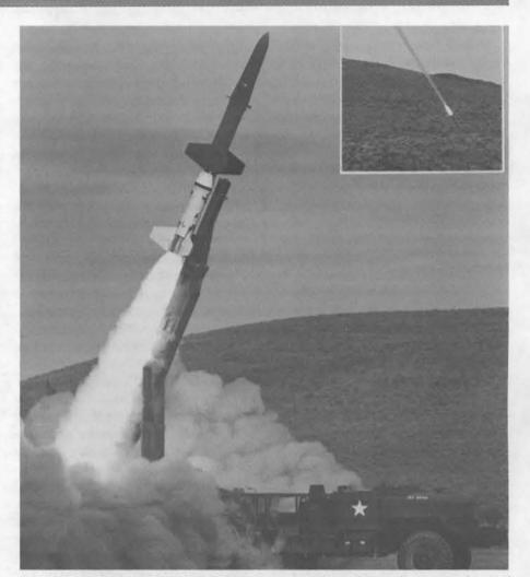
TWO-STAGE GENIE ROCKET SYSTEM was used for a full-scale structural test of a strategic earth penetrator. The first stage lifted the penetrator; the second drove it into the earth at 1460 mph (inset).
