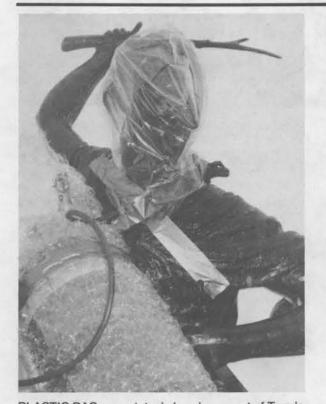
PLASTIC BAG over statue's head was part of Terry's setup for checking whether gypsum could seep out through pores in the bronze.
