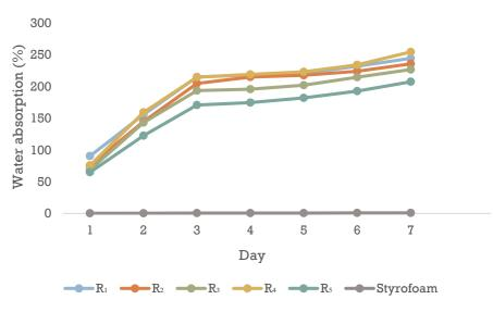
Figure 1. Water absorption behaviour of mycelium biocomposite and styrofoam.
