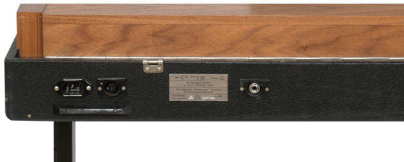
Figure 2: The backside of the instrument with the power supply and the jack plug. Picture Mario Brand 2020
