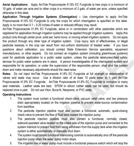
The irrigation line or water pump must include a functional pressure switch which will stop the water pump motor when the water pressure decreases to the point where pesticide distribution is adversely affected.
