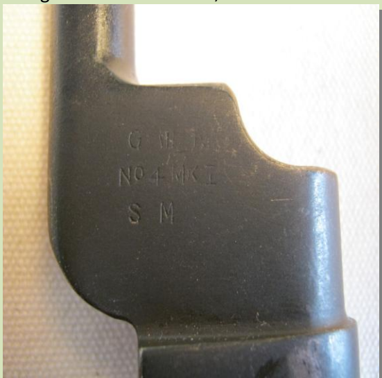
Genuine: note radius on socket & correct marking,
