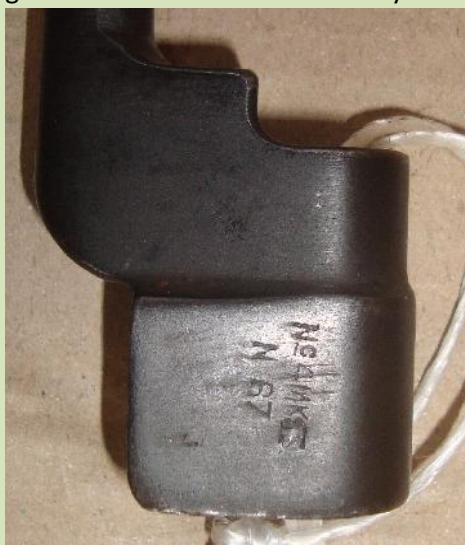
Fake: smaller radius and incorrect marking
