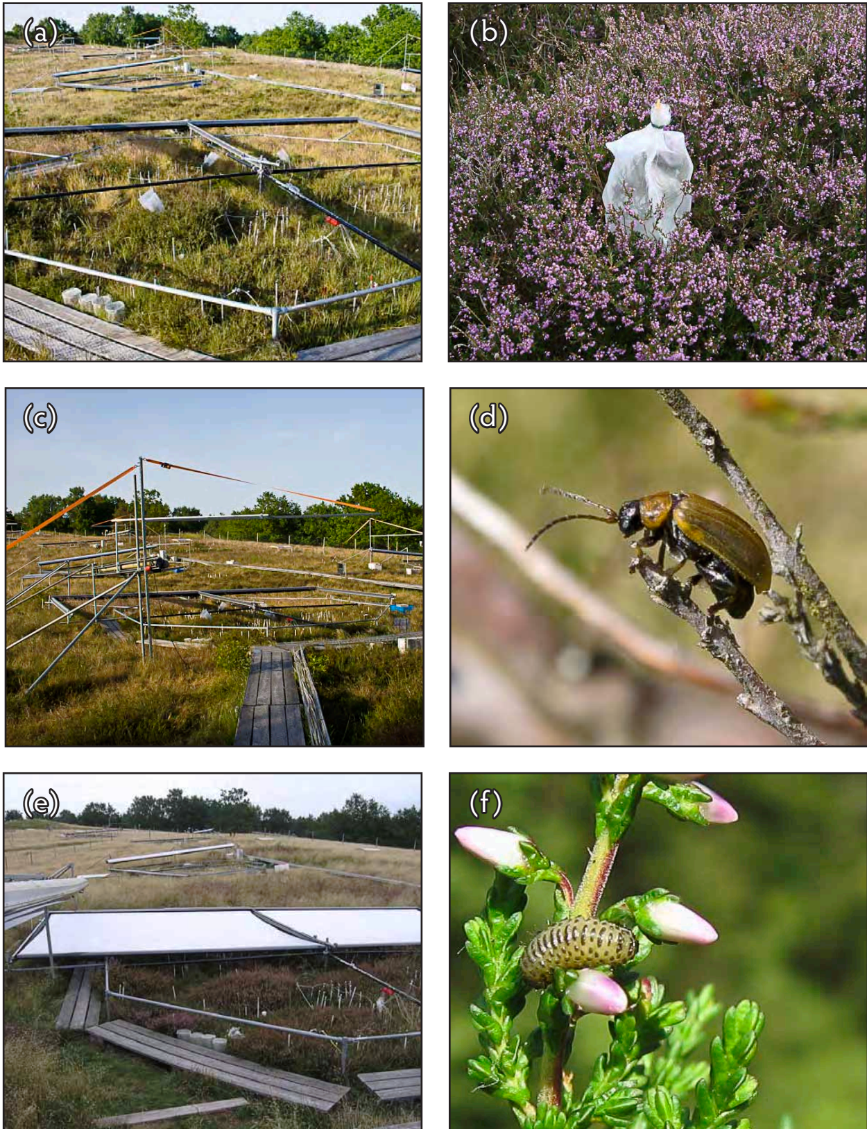
Plate 4 Climate change experiment ("Climaite"), covered in Section 2 of this thesis. (a), (c) and (e) Overview of individual FACE rings (each measuring 7 m in diameter); Each ring is subdivided into four sectors for treatment combinations of drought and warming; (e) a drought curtain moved over half of one of the octagons. (b), (d) and (f): Experiments with the heather beetle, Lochmaea suturalis (see Chapter 5, page 85). (b) Cage stocked with beetle larvae; (d) adult beetle and (f) larval beetle feeding on Calluna vulgaris .
