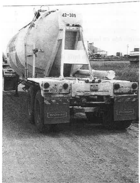
(Above, right) End view of one of the triple-hopper trailers used to carry cement from the plant.
