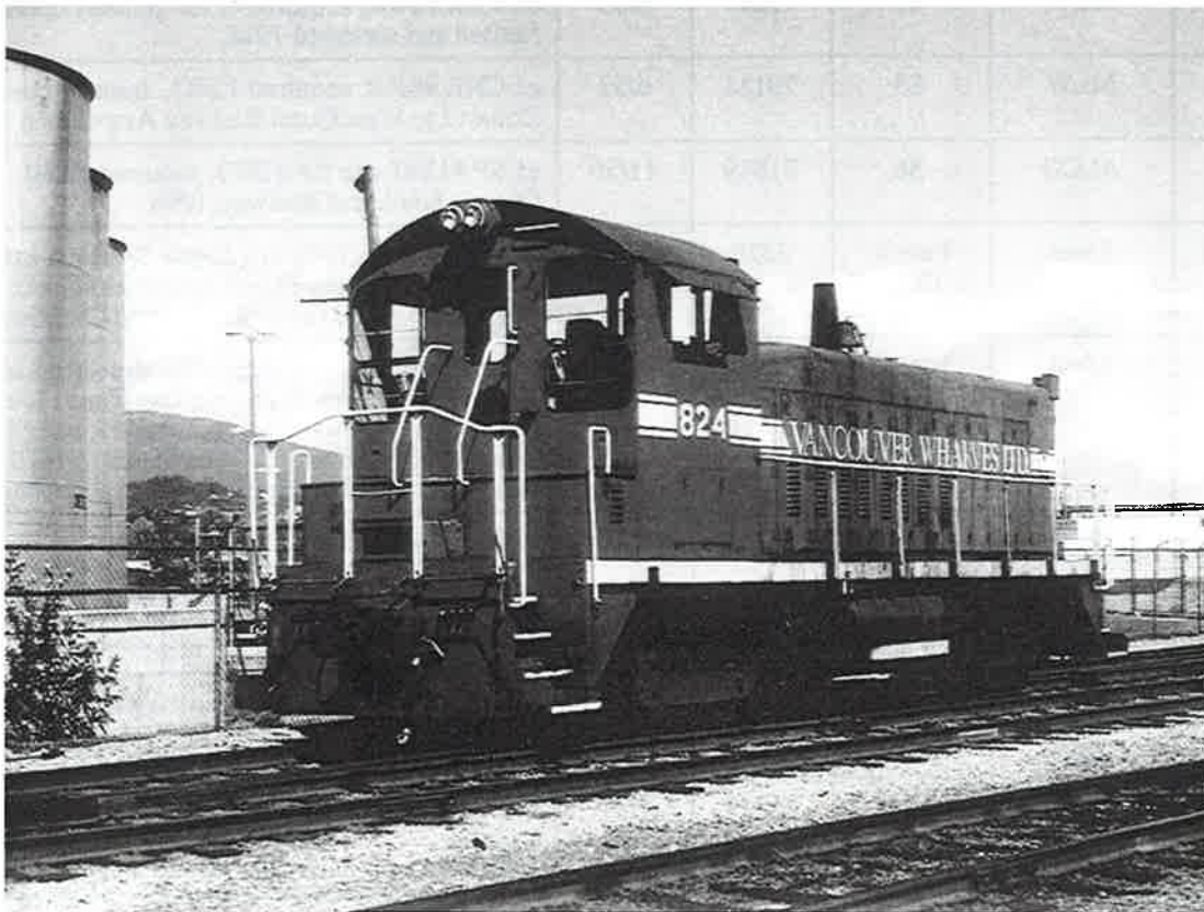
SW1200 #824 was still equipped with Missouri Pacific style classification lights on the front of the long hood and a twin horizontal headlight on the rear of the cab. Photographed by Ron Tuff on June 26 1995.
