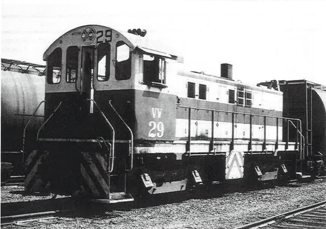
Number 29 was an ALCO S6 #1240 purchased from Southern Pacific in October 1980. It was repainted in the Tacoma Municipal Belt inspired scheme of white with a red stripe and roof. By 1987, it had been repainted red with a white hood stripe. Photographed by Paul J. Crozier Smith on August 17 1981.
