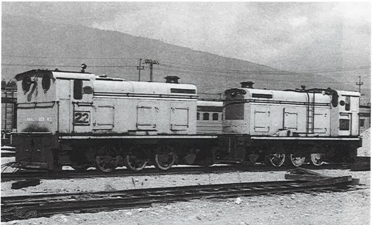
The Hudswell Clarke & Company locomotives arrived in North Vancouver in 1961, painted light blue. The connecting rods and the North American style couplers have not been installed yet. Notice the Pacific Great Eastern passenger equipment in the background. Photographed by Roger F. Behn.
