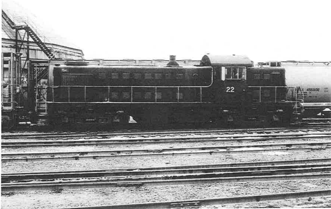
The only non-switcher design locomotive owned by Vancouver Wharves was a RS1 purchased from Atlas Mine & Mill. Painted in the traditional black with yellow railings and cab number, notice the original number 54 still appears in the long hood number board. Photograph by Ron Tuff on May 18 1980.
