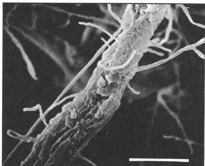
Plate I, Fig. 1. Textile fibre with microorganisms on the surface. Bar = 10 \mu m. Photo V. Kalousková.
