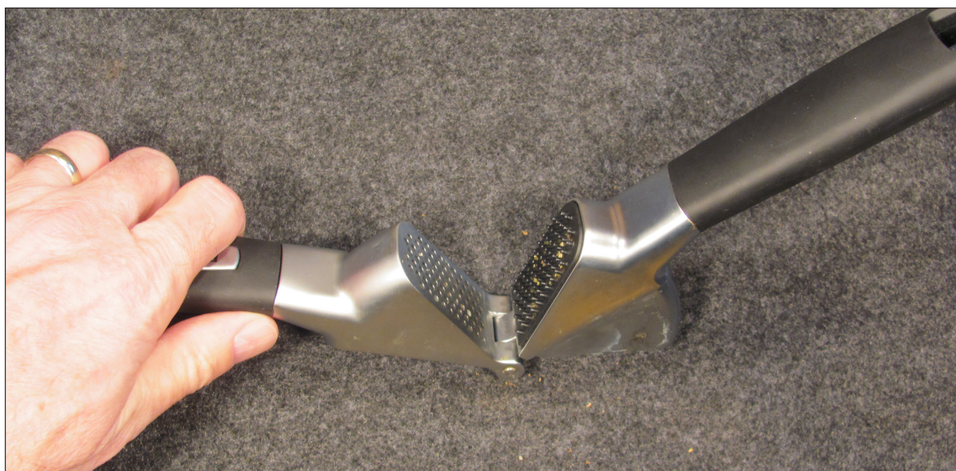
A garlic press may be used to extract sap for petiole testing.
