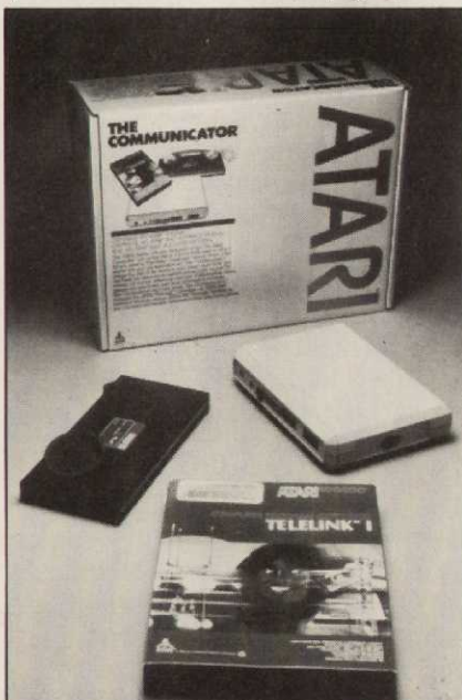
The Communicator Kit provides the Telelink II cartridge and the 835 Direct Connect Modem.
