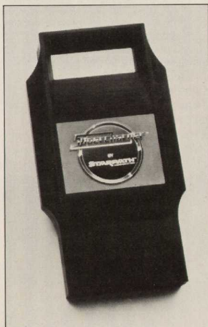
Starpath's Supercharger increases the 2600's RAM capacity fifty times.
