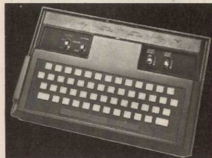
Atari's computer keyboard for the 2600 is inserted in the cart slot.
