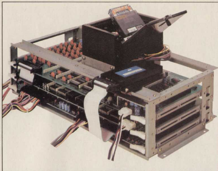
The almighty conversion kit can replace a dying game with a new one in hours. Above is the Data East Multi Conversion Kit with PC boards, cassette deck, control panel graphics and more.
