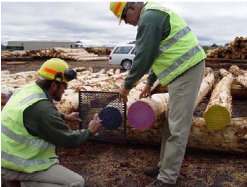
Radiata pine logs are colour coded on the ends with a template to track sawn boards in the mill during processing
