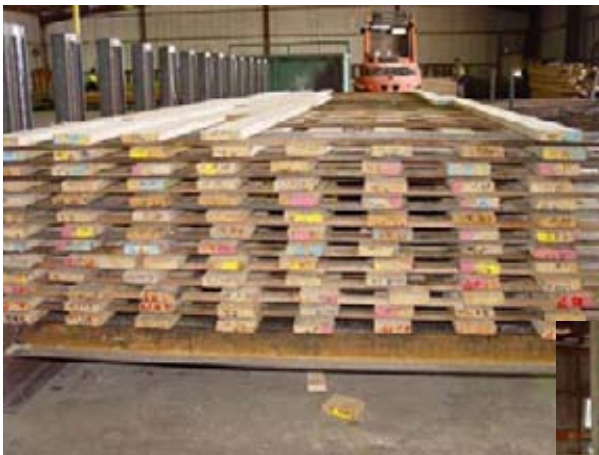
Alpine ash boards being stripped out for air-drying at Neville Smith Timbers at Seymour, Victoria
