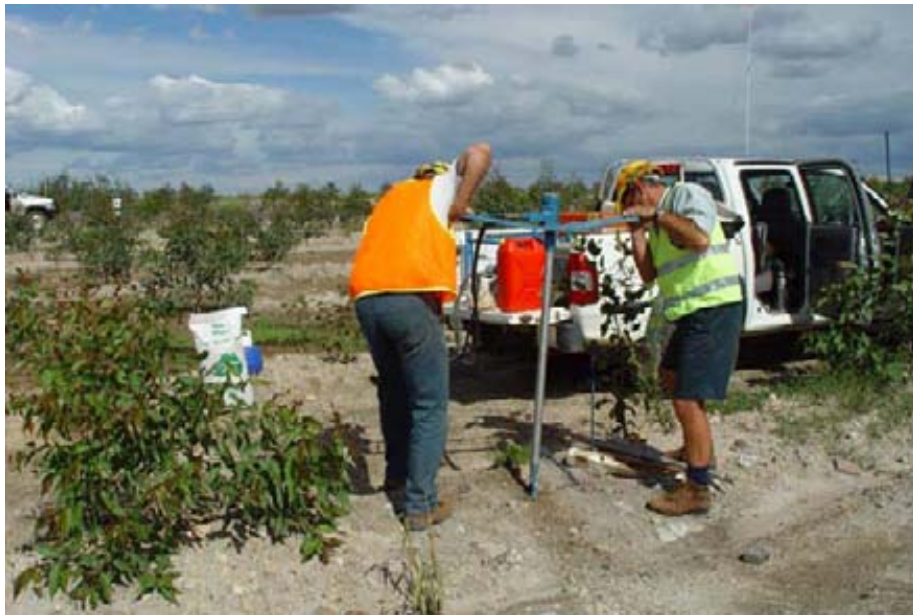
Installing Neutron Probe access tubes to monitor soil moisture
