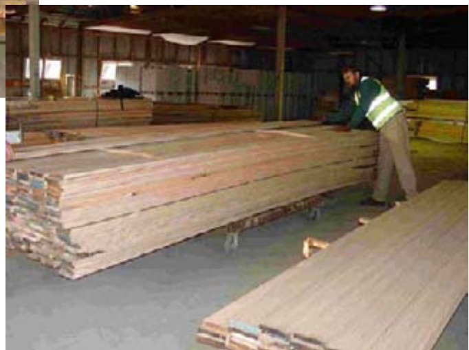
Grading of alpine ash boards for appearance products after kiln drying and dressing at Neville Smith Timbers at Seymour, Victoria
