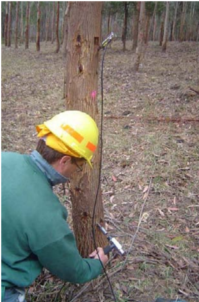
Acoustic tool used for assessing wood quality in a six-year-old clonal Eucalyptus pilularis (blackbutt) trial
