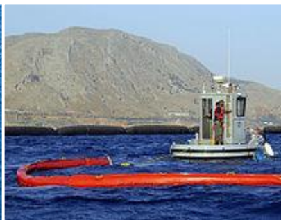
Illustration 10.2.10h: A U.S Navy oil spill response team drills with a "Harbour Buster" high-speed oil containment system".
