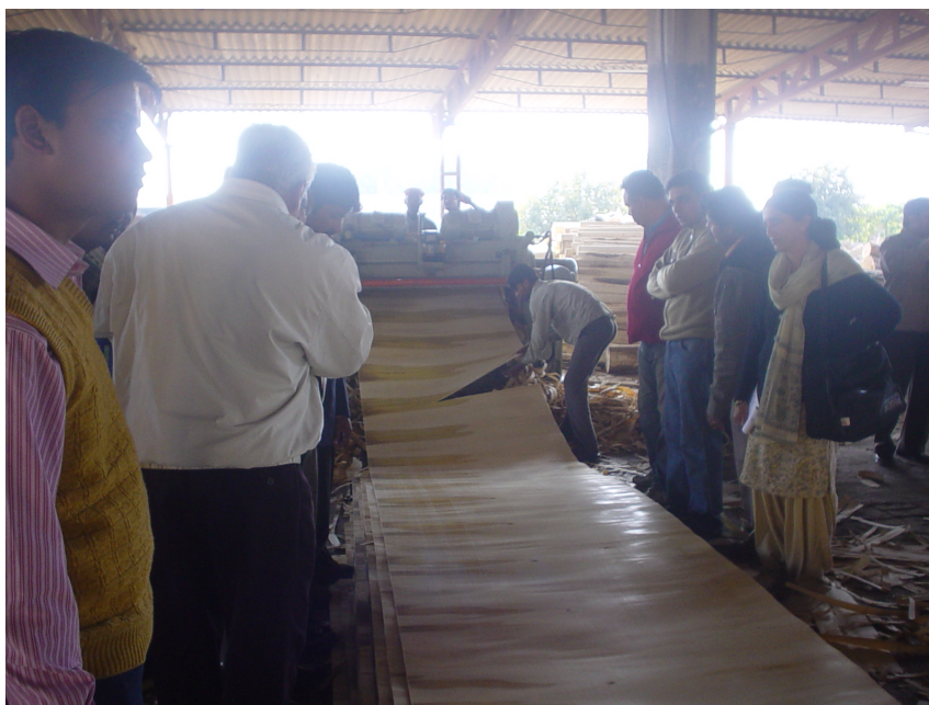
Fig. 1.14: Peeling of poplar logs for plywood production, northern India. Photograph: Chauhan, pers. comm.
