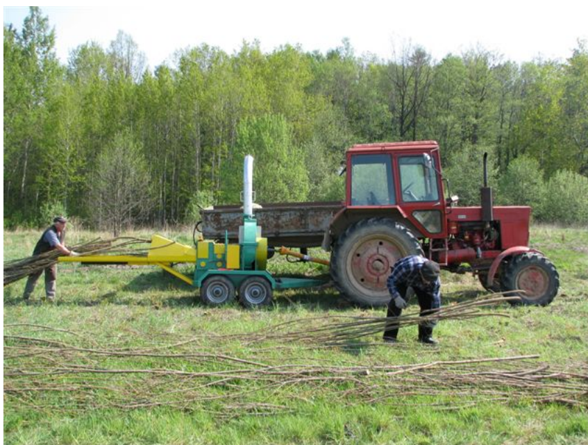
Fig. 1.12: Mobile chipper, here used for willow in Poland. At the left the driver of the tractor helps with chipping. One person also working on the field is not visible. The total team is three persons (1 driver and two workers). Photograph: Jan Dubas, Poland
