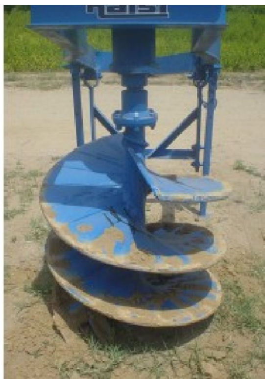
Fig. 5.3: Tractor mounted auger for digging pits.
