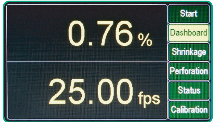
2: The Dashboard tells you the shrinkage measured at that instant, and the film frame rate at that moment.
