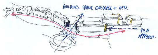
The curved form relates to the site and movement paths as well as view corridors where the buildings peel into or out of view. The nature of this curve groups the buildings together as a family, and as such we see a common language of components which can be used across all the buildings. This provides the development a cohesive appearance, yet the language can be expressed in varying ways so as to allow for individual expression where required.
