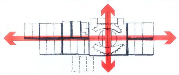
The strong east-west axis of the ladder establishes a clear differentiation between front-of-house activities and back-of-house activities. The orientation of the courts is also designed to minimise glare and wind tunnelling.
