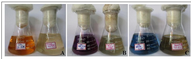
Fig.3: Degradation of Azo dyes by Trimmatostroma sp. A) Congo red, B) Crystal violet and C) Remazol brilliant blue (25 \mu g/mL). The two flasks in each panel represent the dyes on 1 st day and after degradation at the end of the 7 th day.
