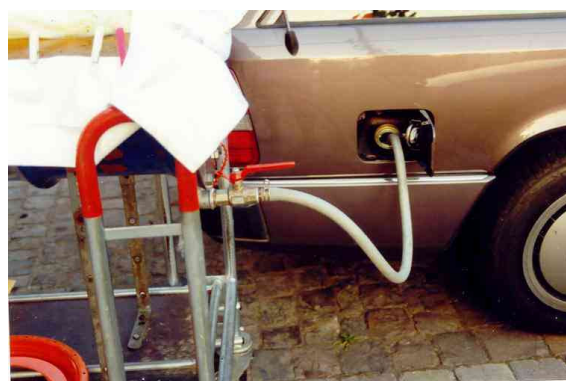
Figure 9 – PPO filtration (in this case used cooking oil) on the site of Monopoeel, http://www.monopoeel.de/stammseiten/eigenes_altp.html . In this case two clothes are used but that is not necessary, one 1 µm cloth is sufficient.
