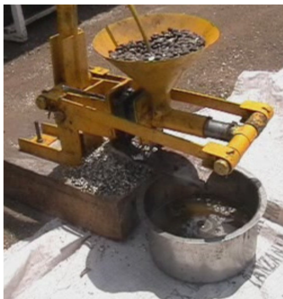
Figure 2 – close-up of the Bielenberg pressing mechanism. Notice the automatic discharge of the pressing chamber and the stopper in the seed funnel [3]
