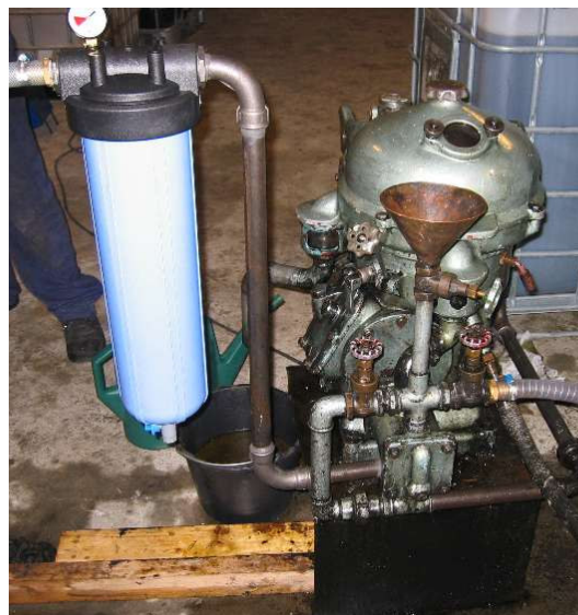
Figure 8 – example of a centrifugation system with a bag filter as a security. [5]
