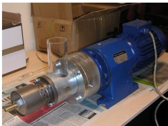
Figure 5 – The Danish BT press is an example of a hole cylinder type press. Notice the nozzle, left in front. [4]
