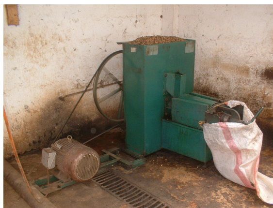
Figure 6 – The Sundhara oil expeller is a representative of the strainer type presses. On the right side the choke adjustment. [3]
