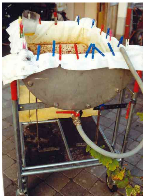
Figure 9 – PPO filtration (in this case used cooking oil) on the site of Monopoeel, http://www.monopoeel.de/stammseiten/eigenes_altp.html . In this case two clothes are used but that is not necessary, one 1 µm cloth is sufficient.
