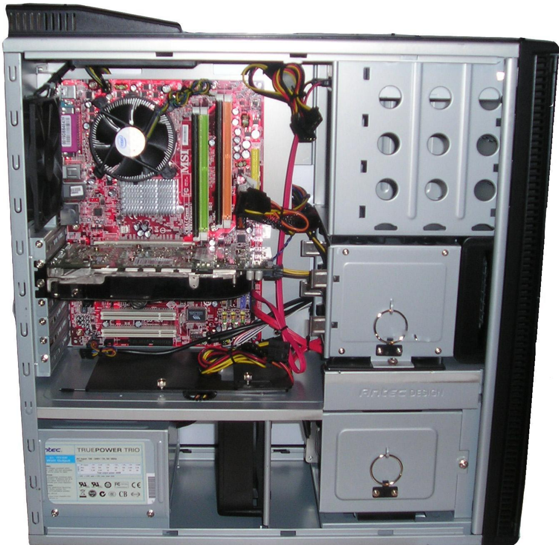
Inside a custom-built computer: power supply at the bottom has its own cooling fan
