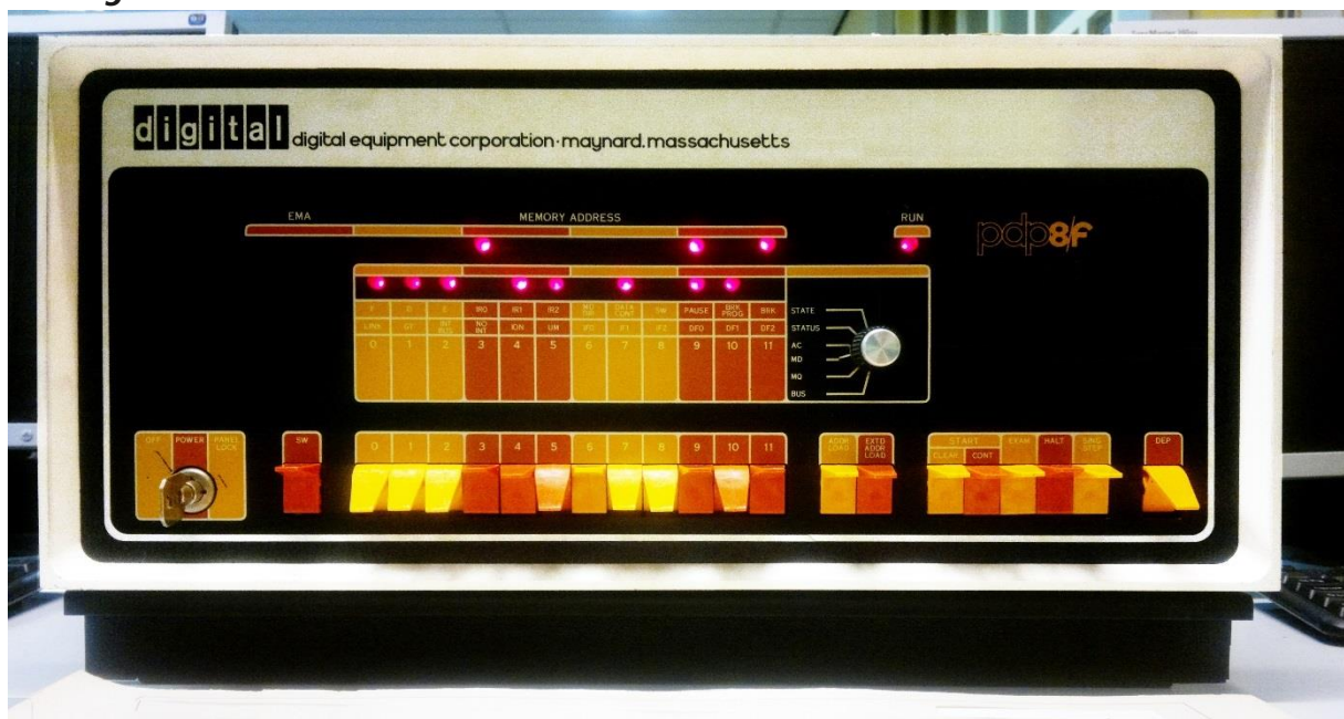
Front panel of an early minicomputer, with switches for entering machine code
