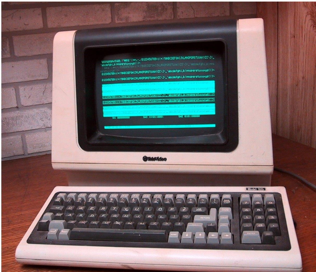
Time-sharing computer terminals connected to central computers, such as the TeleVideo ASCII character mode smart terminal pictured here, were sometimes used before the advent of the PC.
