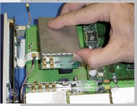
Moreover, the outstanding feature that service can be easily done by simply replacing plug-in pre-calibrated subassemblies, represents a highly valued advantage in case, for example, of damage to the RF front-end. Indeed, even when an excess of energy
