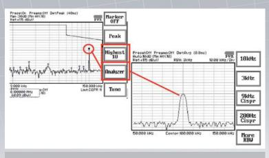
The 9010 features several useful functions: as an example, pictures above show the automatic highest peaks finder and the intuitive way to observe the selected peak in Analyzer mode: from measurement to debugging at users' fingertips!
