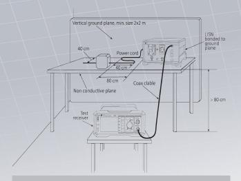
Example of Test Setup for RFI Voltage Measurement
