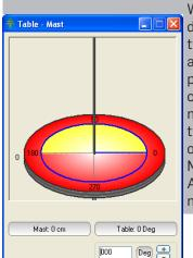
When debugging the antenna and turntable positioning can be set manually and the receiver operated in Manual and Analyzer modes.
