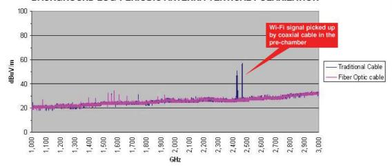
Comparison between antenna-receiver connected by coaxial cable (blue trace) and 9030 directly connected to the antenna and linked to 9010 by fiber optic cable (pink trace).
