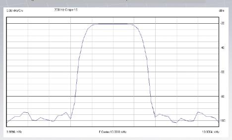
After the A/D conversion the behaviour of a regular receiver is mathematically simulated in order to perfectly match international standards specifications. Even for a digital architecture, preselector filters and input attenuators are mandatory for limiting the signal energy into well defined RF bands, to improve the dynamic range and to increase the signal to noise ratio, thus ensuring accurate measurements of all wideband complex signals typical of EMC measurements.
