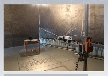
Radiated measurements with 9030/9060/9180 mounted directly on an antenna connector
