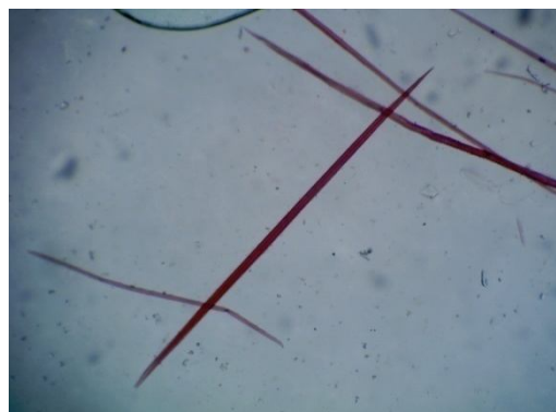
Figure2. View of fibre of Bamboosa garuchakoa under microscope (10X magnification)
