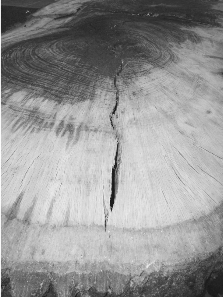
The slice has started to check, but not as badly as expected given 6 months of preparation and drying time. photo©Zarah Wyly
