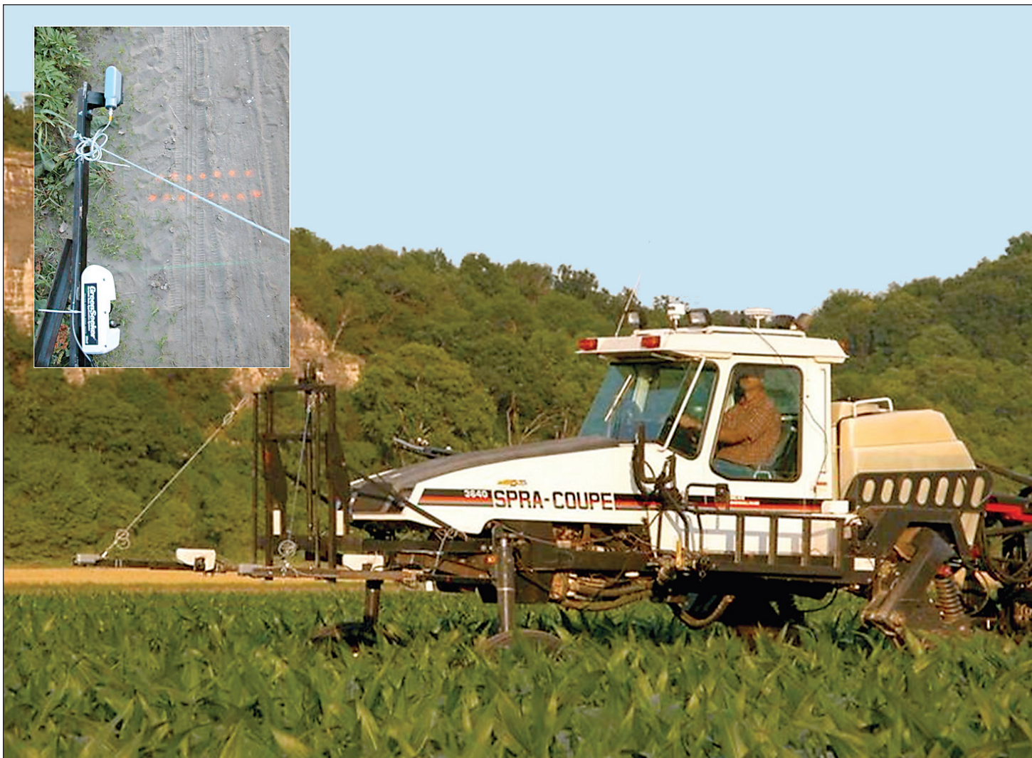
A high clearance vehicle equipped with active-light reflectance sensors to guide in-season N application. Inset: The Holland Scientific Crop Circle™ ACS-210 Sensor (top) and NTech Industries GreenSeeker® Sensor (bottom) project their corresponding light pattern onto the soil surface.
