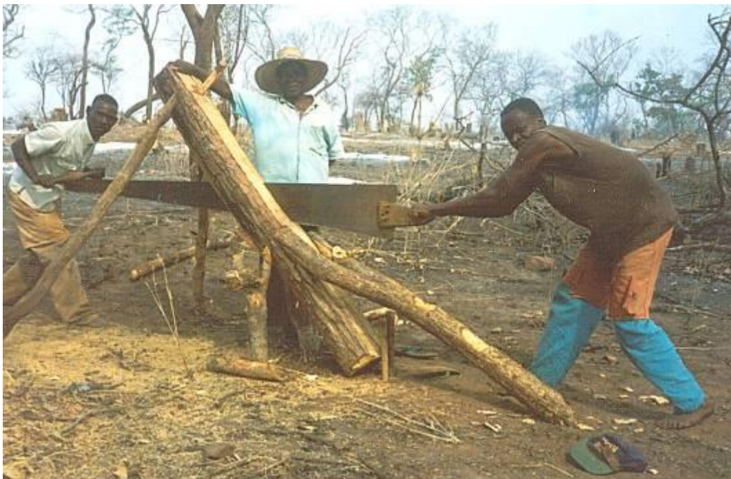
Pitsawing is an ecologically sound way to make planks from trees.
