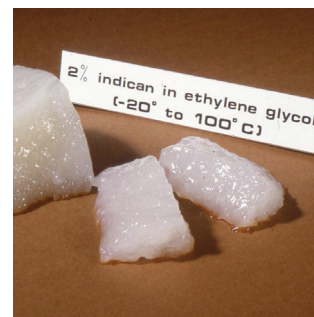
Fig 35 Polysaccharide gel formed with ethylene glycol as solvent
