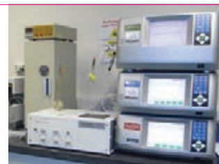
Fig 24 Size exclusion chromatography with multi-angle light scattering equipment
