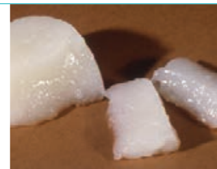
Fig 86R Indican gel formation in ethylene glycol
