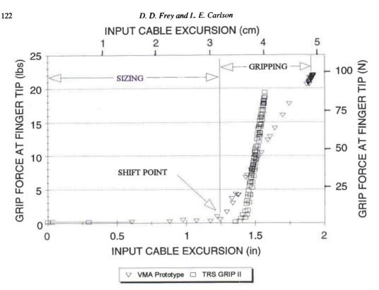
Fig. 6. Sensitivity of the VMA prototype and TRS GRIP II to errors in input cable excursion.
