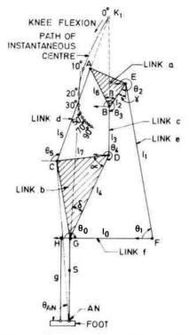
Fig. 2 Six-bar linkage knee-ankle mechanism used in the new prosthesis
