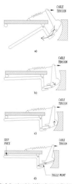
Fig. 2. Operation of the VMA prehensor, a) The VMA prehensor sizing an object b) When an object is met, the mechanism shifts into high mechanical advantage operation. The input lever comes into contact with a quadrant, c) In high mechanical advantage operation, the lever rolls along the quadrant, d) Finally, the mechanism reaches a toggle point and a holding assist function is activated.
