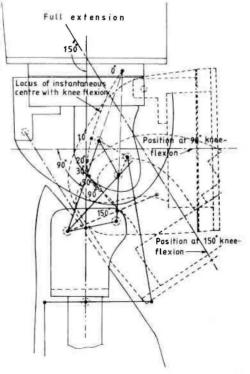
Fig. 3. Locus of instantaneous knee centre for rotation of thigh relative to shank up to 150° of flexion.
