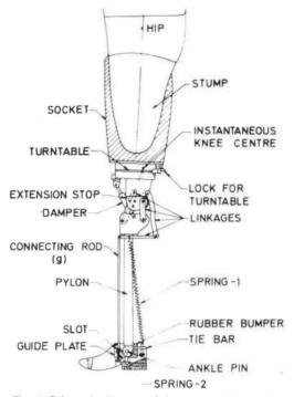
Fig. 1. Schematic diagram of the new modular six-bar linkage trans-femoral prosthesis.
