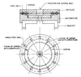
Fig. 5. Details of turntable used for cross-legged sitting.
