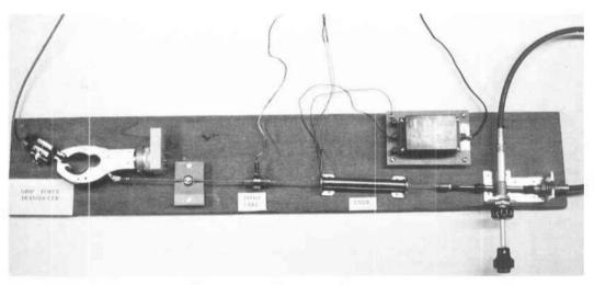
Fig 4. The grip performance testing apparatus
