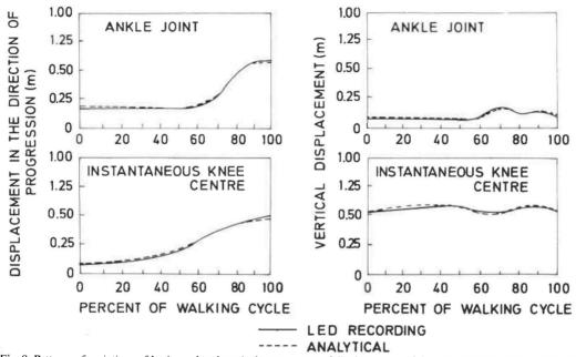
Fig. 9. Patterns of variations of horizontal and vertical components of displacements of the instantaneous knee centre and the ankle joint
