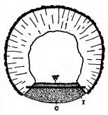
FIG. 52. — Illustrating cross-section of the cement snrface covering to cavity shown in Fig. 51. W, wire stapled to sides of cavity; I, iron re-enforcing; C, cement.
