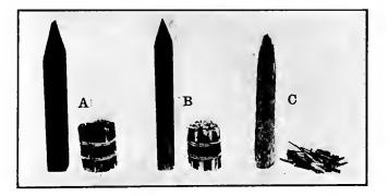
FIG. 26. — Effects of antiseptic treatment of wood in soll two years: (a) treated with Carbolineum; (b) creosote; (c) untreated. Little difference between (a) and (b); in (c) practically all decayed and about 50 per cent. completely.
