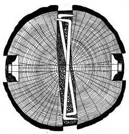
FIG. 45.— Cross-section of split tree with bolt and countersunk nuts and washers and Iron braces to obviate movement. Instead of cement, wooden hlocks should be employed to cover the opening of the cavity.
