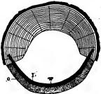
FIG. 55. — Section of tree with cavity illustrating wire and elastic cement method of covering openlog. C, elastic cement; W, wire mesh; I, iron re-enforcements.
