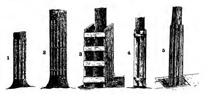
FIG. 58. — Different types of tree guards: 1, wooden strips nailed to a tree; 2, wooden strips nalled to a tree and banded with iron; 3, old type of wooden tree guard;
