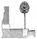
FIG. 16 — Illustrating method of growing trees on busy thoroughfares. The conventional type, such as the Oriental plane which tolerates severe annual pruning, is planted between the sidewalk and curbing in a rich loam 3 or 4 feet deep, provided with special subirigation tile.
