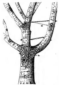
FIG. 32. — Improper method of chaining tree. Dotted lines show more effective method: (b) bolt, (c) chain. All chains, however, too low.
