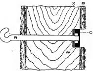
FIG. 35. — Longitudinal section of limb, showing method of bolting. B, hark; X, wood; R, holt; W, washer; C, cement.
