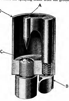
FIG. 109. — "M. A. C." nozzle. A, atomizing point or deflector; B, wing handle to adjust or swing point; C, nozzle proper; D, hollow case to protect A and C.
