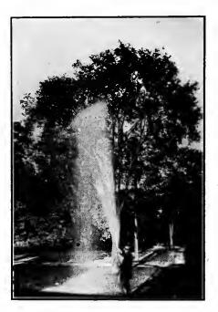
FIG. 108. — "M. A. C." nozzle spray with highpressure and atomizing point intercepting the stream.
