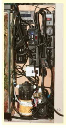
THE automated control for the terrarium's temperature and humidity is based on the Digital Aquatics HerpKeeper system and is mounted on a wood board with all components and wires labeled.
