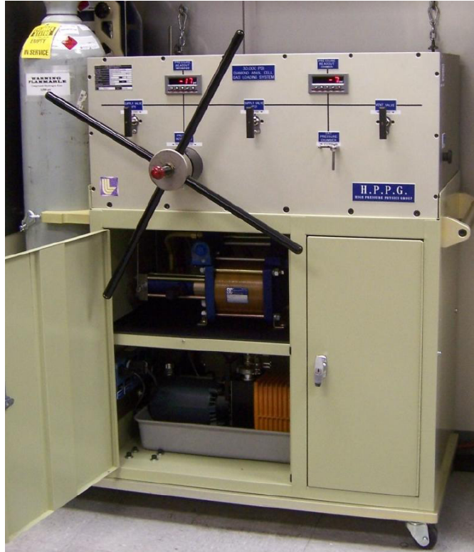
Figure 4.7. 30,000 psi high pressure gas loader. Gas is loaded from the cylinder (closed in this image) into the loader, and the pressure within is increased little by little, by turning the pressure intensifier ([mechanical name for the PI]).
