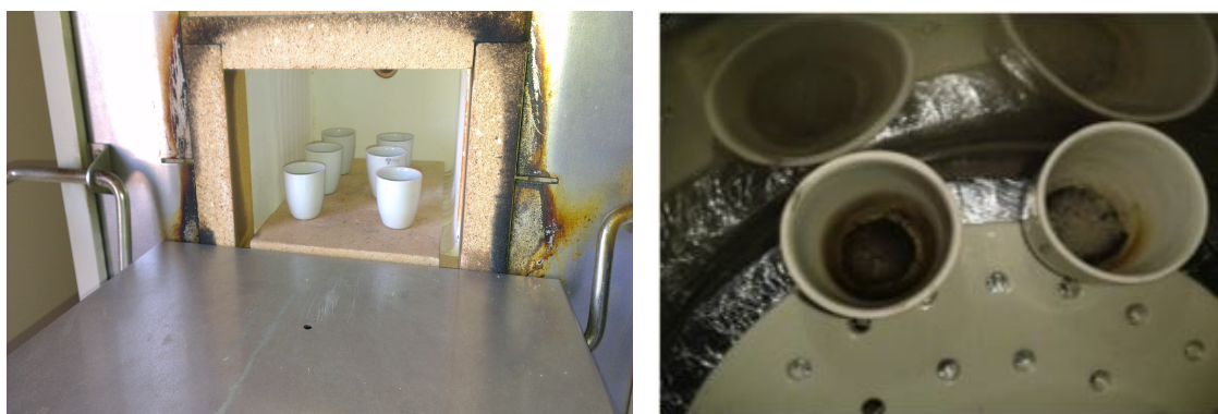
Figure 3.3. Crucible and samples of peppermint and basil in to the burner oven to measure and calculate ash for experimental plants in this study.
