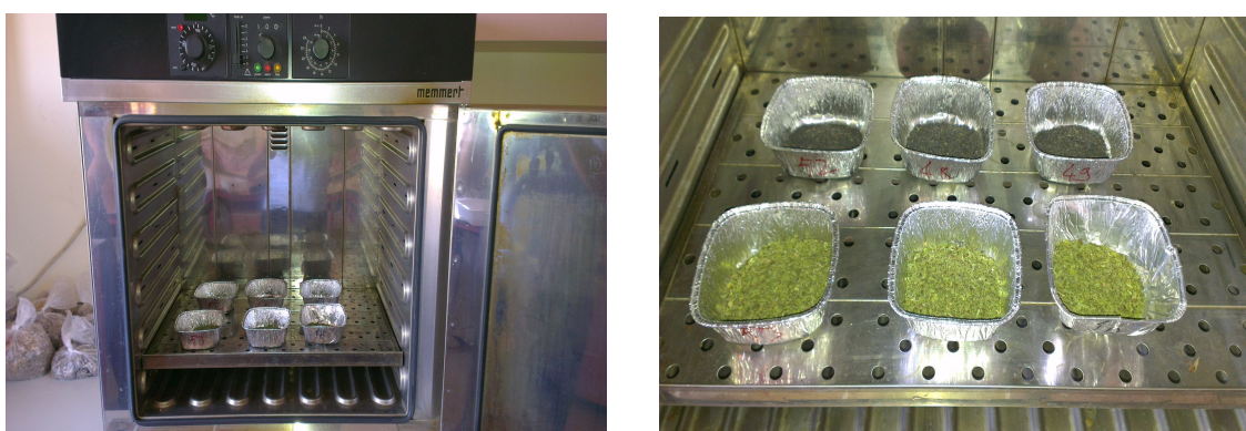
Figure 3.2. Sample of peppermint and basil on the electrical oven to measure and calculate dry matter in this study.
