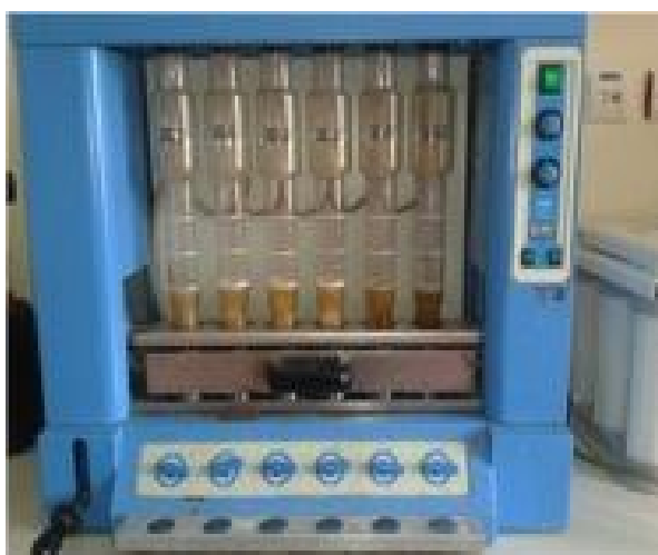
Figure 3.6. Measure and calculate crude fiber in the peppermint and basil by using NDF-boiling apparatus in this study.
