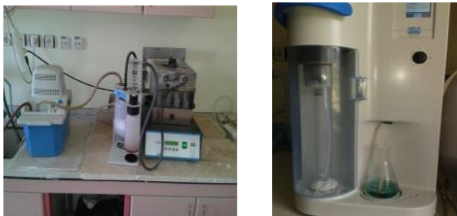
Figure 3.4. Kjeldahl method and flasks to digest protein in the peppermint and basil in this study and calculate crude protein.
