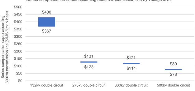
Series compensation capex assuming 300km transmission line by voltage level
