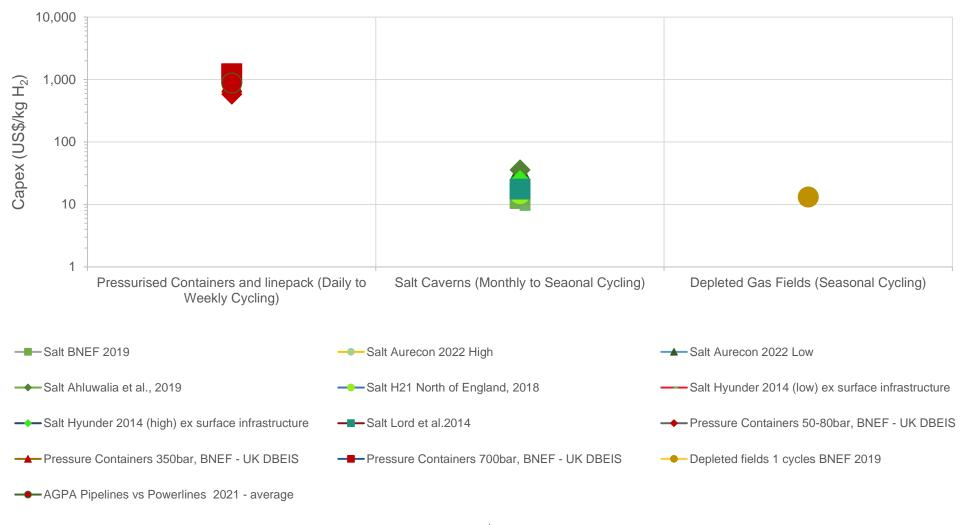
Figure 22: Hydrogen gas storage costs for different storage types (capex per kilogram H<sub>2</sub>). Current prices (2019-22)
