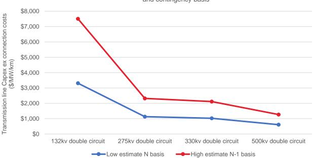
Transmission line capex (ex terminal stations and series compensation) per voltage and contingency basis
