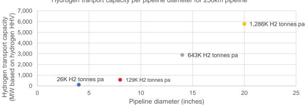
Hydrogen tranport capacity per pipeline diameter for 250km pipeline
