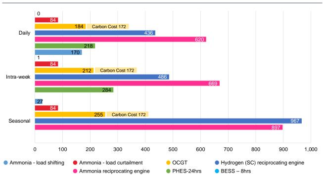
2040 - Levelised cost excluding carbon costs by Cycling Interval - 2040 (\$/MWh)
