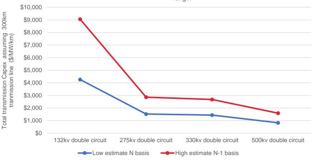
Total transmission capex per voltage and contingency basis assuming 300km line length
