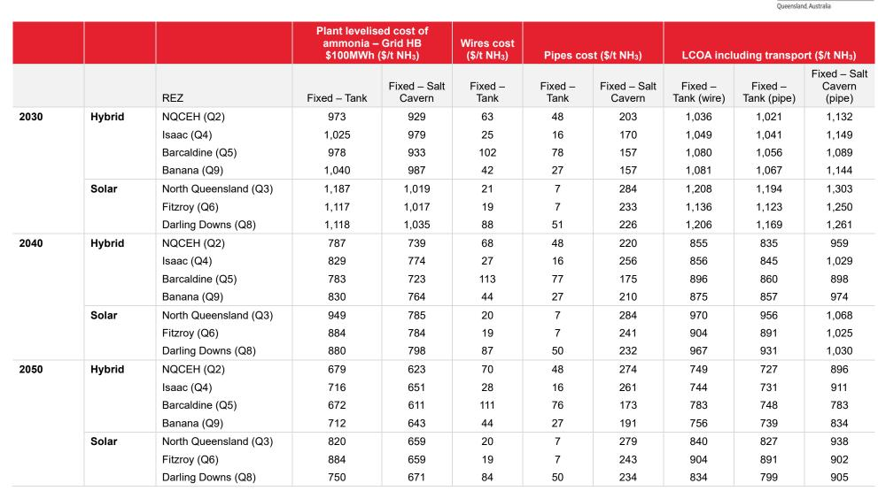
Table 10: LCOA including transport – Grid connected HB paying \$100MWh by scenario and REZ all years
