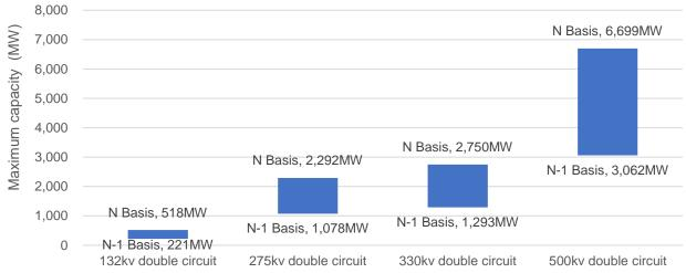
Figure 36: Double circuit line capacity and voltage level Data source: 2022 AEMO Transmission Cost Database (2023).
