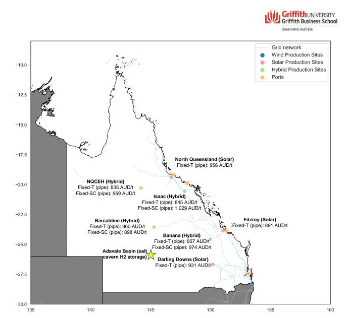
Figure 45: Map showing selected 2040 LCOA (\$/t NH<sub>3</sub>) including transport – Grid connected HB paying \$100MWh for selected scenarios
