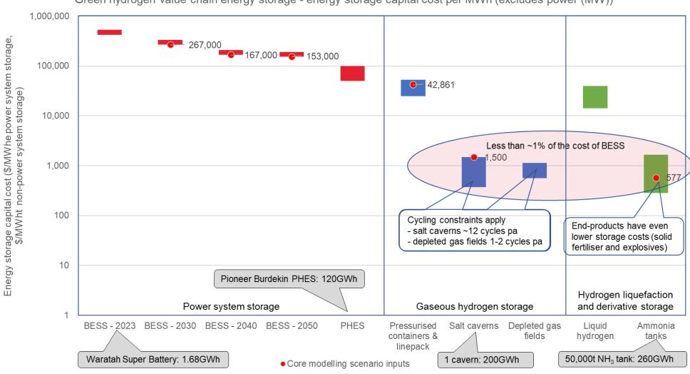
Green hydrogen value chain energy storage - energy storage capital cost per MWh (excludes power (MW))
