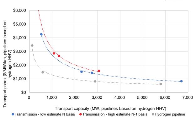
Figure 30: Capex vs. capacity for 250km transmission and one way hydrogen pipelines
