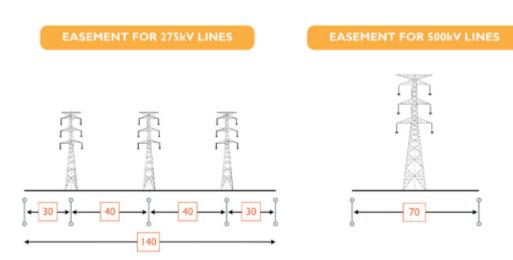
Figure 38: Easement widths Source: Powerlink (2022)
