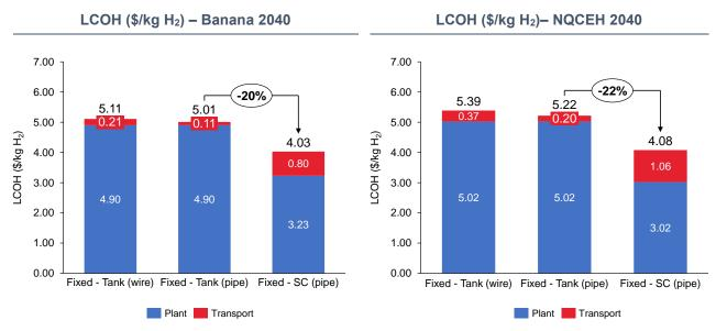
Figure 42: LCOH including transport in the different scenarios at Banana 2040 (left) and NQCEH 2040 (right)
