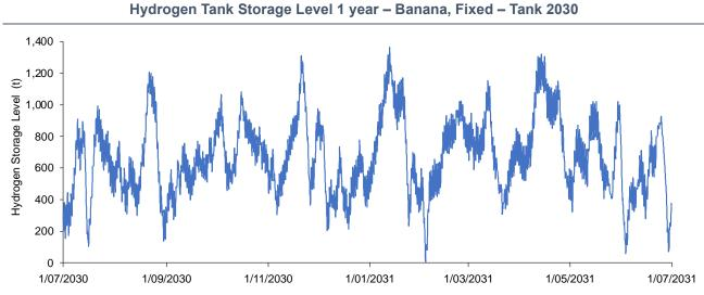
Figure 22: Hydrogen – level of hydrogen storage in hydrogen tanks over one year at Banana (Fixed – Tank) 2030
