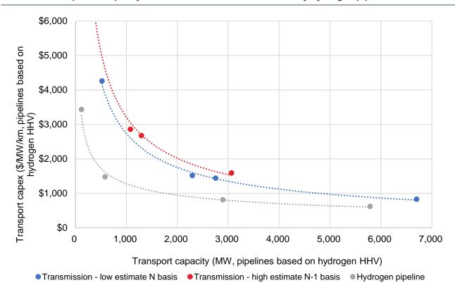
Capex vs capacity for 250km transmission and one way hydrogen pipelines
