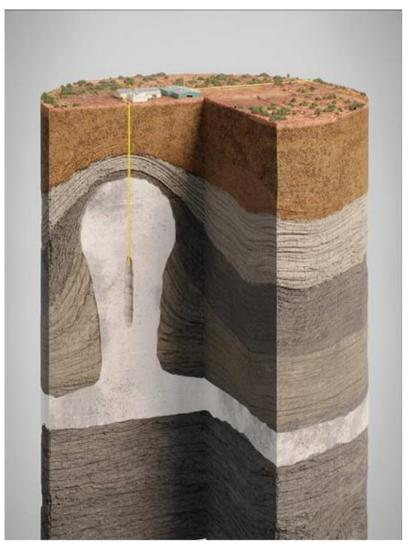
Figure 24: Salt cavern cross section Source: Geoscience Australia (2022).
