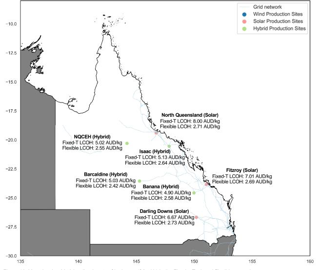
Figure 16: Map showing 2040 levelised costs of hydrogen (\$/kg H<sub>2</sub>) in the Fixed – Tank and Flexible scenarios
