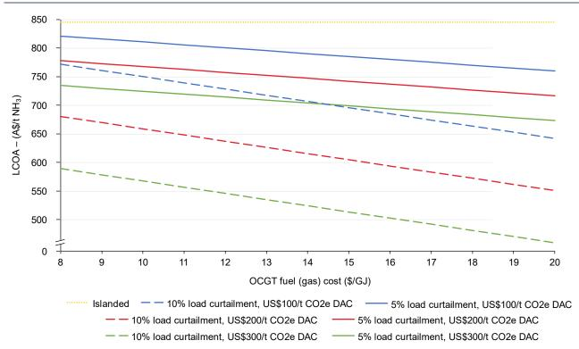
Figure 60: LCOA including load curtailment: Isaac – Fixed-Tank, grid connected HB at \$100Mwh, H2 pipes transport (A\$/t NH<sub>3</sub>)
