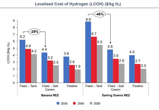
Figure 15: Levelised Cost of Hydrogen (LCOH) under different scenarios in different years in Banana and Darling Downs (solar PV only).
