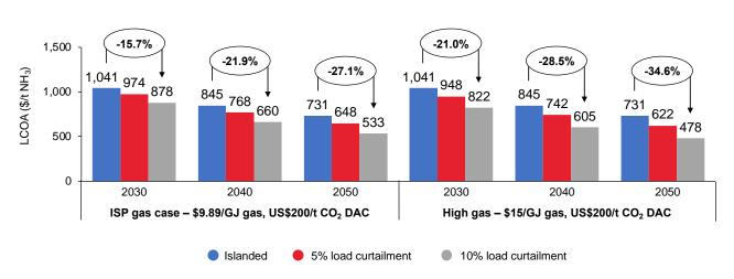
Figure 59: Demand response impact on LCOA: Isaac – Fixed, H2 pipes transport (A\$/t NH<sub>3</sub>)
