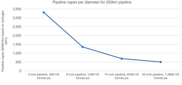
Figure 32: Pipeline capex per diameter for 250km pipeline Data source: Australian Gas and Pipeline Association. (2021).
