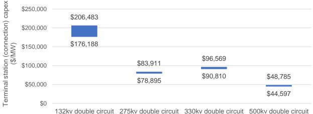
Figure 40: Terminal station (connection) capex for both ends of transmission line by voltage level
