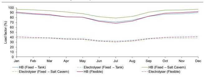
Figure 35: Ammonia – average monthly ammonia plant and electrolyser load factors for three scenarios in Banana
