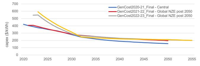
Figure 2: CSIRO GENCOST 4 hr BESS capex (Step Change)
