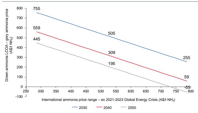
Figure 47: Green ammonia green premium: Isaac – Fixed – Tank, Grid connected HB at \$100MWh, H<sub>2</sub> pipes transport (A\$/t NH3)
