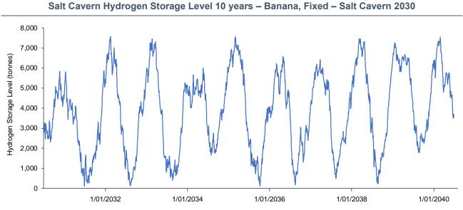
Figure 24: Hydrogen – level of hydrogen storage in Fixed – Salt Cavern case over 10 years (2030-2040) at Banana
