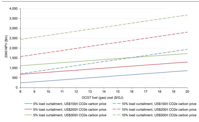
Figure 61: System cost benefit of load curtailment: Isaac 2040 – Fixed-Tank, Grid connected HB at \$100MWh,  $H_2$  pipes transport (A\$/t NH<sub>3</sub>)
